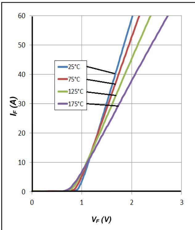
Figure 1. Forward Characteristics
