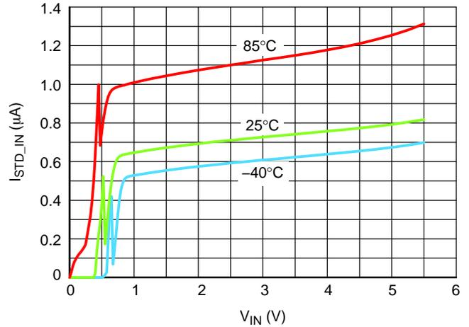
Figure 7. Standby Current (µA) vs. V<sub>IN</sub>, Multi Junction Temperature
