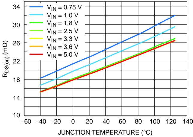
Figure 6. R<sub>DS(on)</sub> vs. Temperature, Multi V<sub>IN</sub> Voltage
