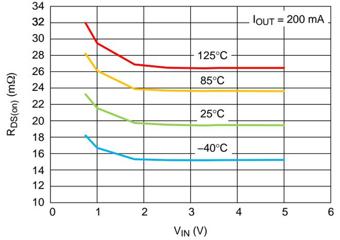
Figure 5. R<sub>DS(on)</sub> vs. V<sub>IN</sub>, Low Load, Multi Junction Temperature
