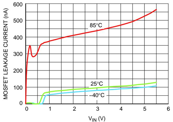
Figure 9. MOSFET Leakage Current (nA) vs. V<sub>IN</sub>, Multi Junction Temperature
