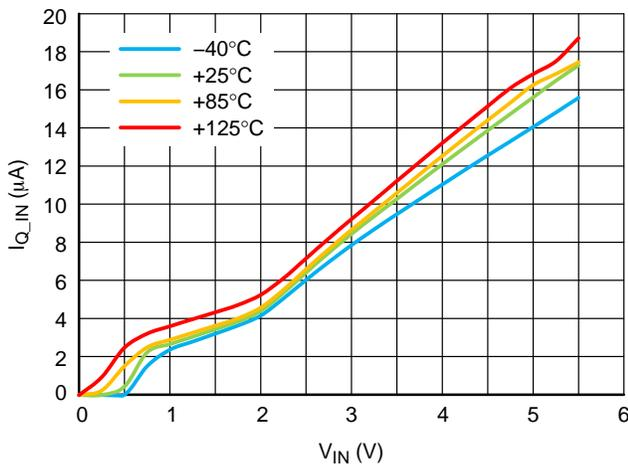
Figure 8. Quiescent Current (µA) vs. V<sub>IN</sub>, Multi Junction Temperature
