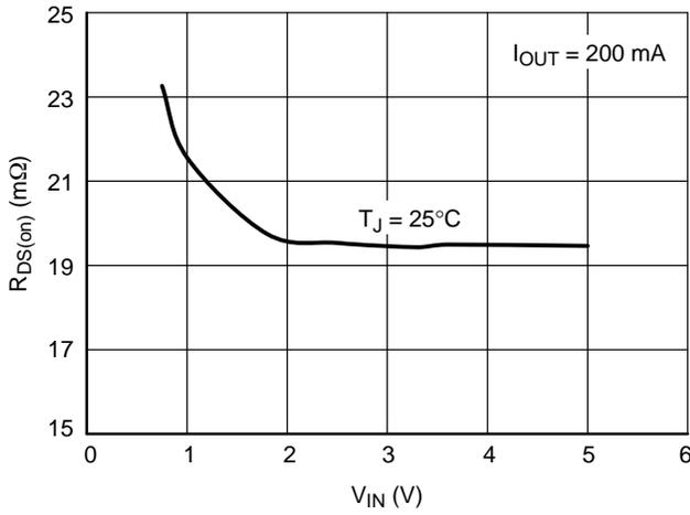
Figure 4. R<sub>DS(on)</sub> vs. V<sub>IN</sub>, Low Load
