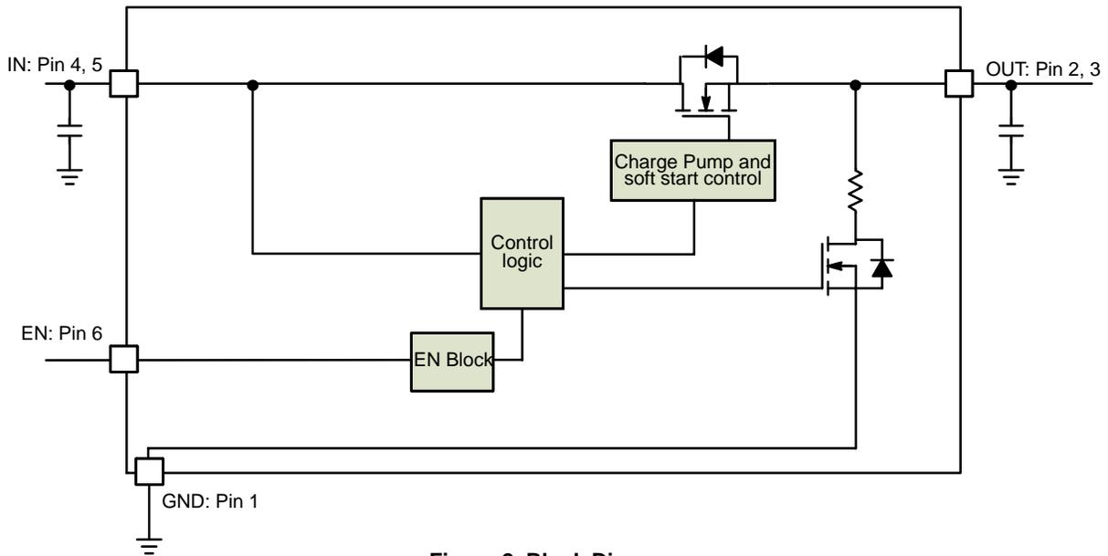
Figure 2. Block Diagram
