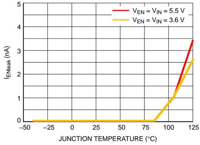
**Figure 10. EN Pin Leakage vs. Junction Temperature**
