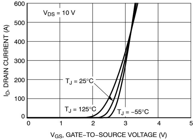
Figure 2. Transfer Characteristics
