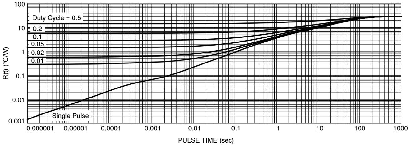
Figure 13. Thermal Characteristics
