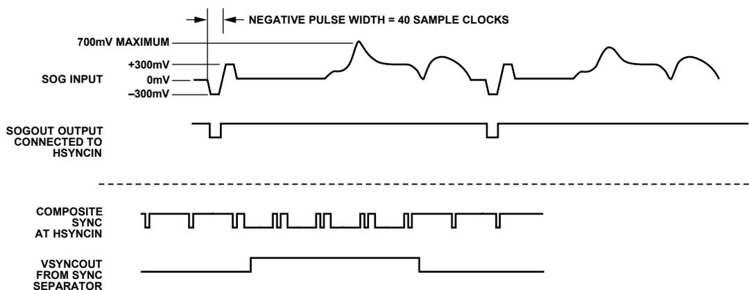
Figure 10. Sync Slicer and Sync Separator Output
