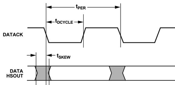
Figure 14. Output Timing
