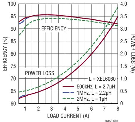
**12V<sub>IN</sub> to 3.3V<sub>OUT</sub> Efficiency vs Frequency**
