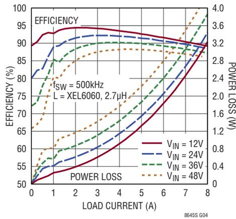
**LT8645S Low Load Efficiency at 5V<sub>OUT</sub>**
