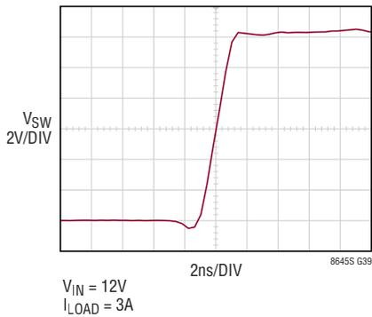
**Switching Waveforms, Full Frequency Continuous Operation**
