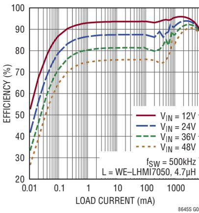
**LT8646S Low Load Efficiency at 5V<sub>OUT</sub>**
