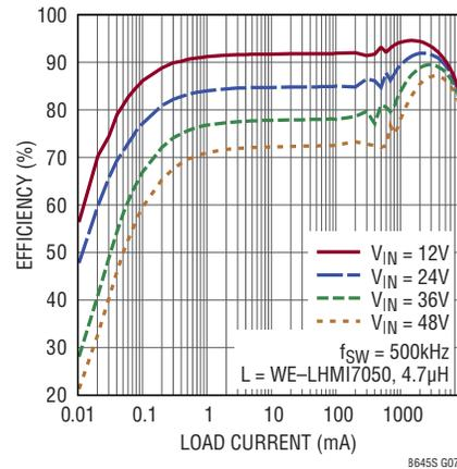
**LT8646S Low Load Efficiency at 3.3V<sub>OUT</sub>**
