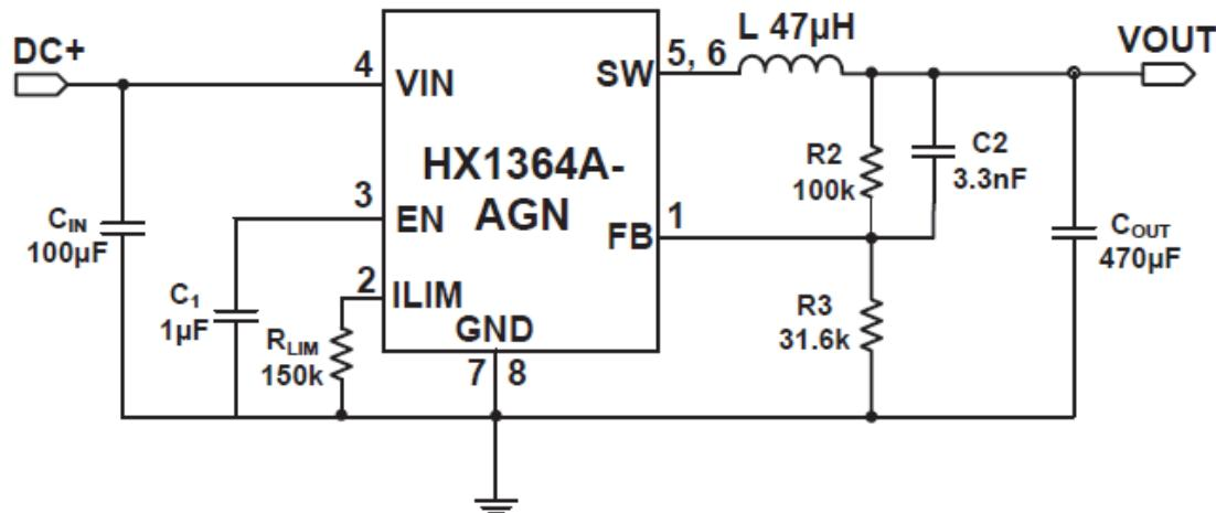
\* The output voltage is set by R<sub>2</sub> and R<sub>3</sub>:  $V_{OUT} = 1.20V \cdot [1 + (R_2/R_3)]$ .
