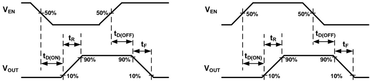
Figure 1. Voltage Waveforms: AP2181D (Left), AP2191D (Right)
