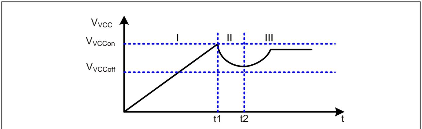
Figure 4 VCC voltage at start up
