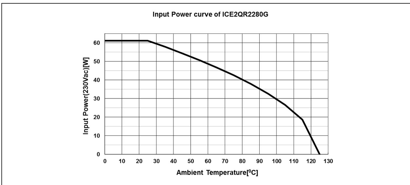
Figure 14 Input power curve  $V_{IN}=230 V_{AC}$ ;  $P_{in}=f(T_a)$
