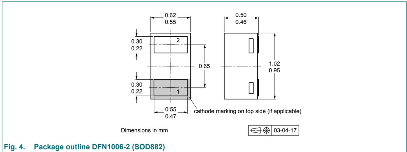
Fig. 4. Package outline DFN1006-2 (SOD882)
