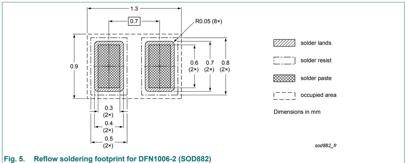
Fig. 5. Reflow soldering footprint for DFN1006-2 (SOD882)
