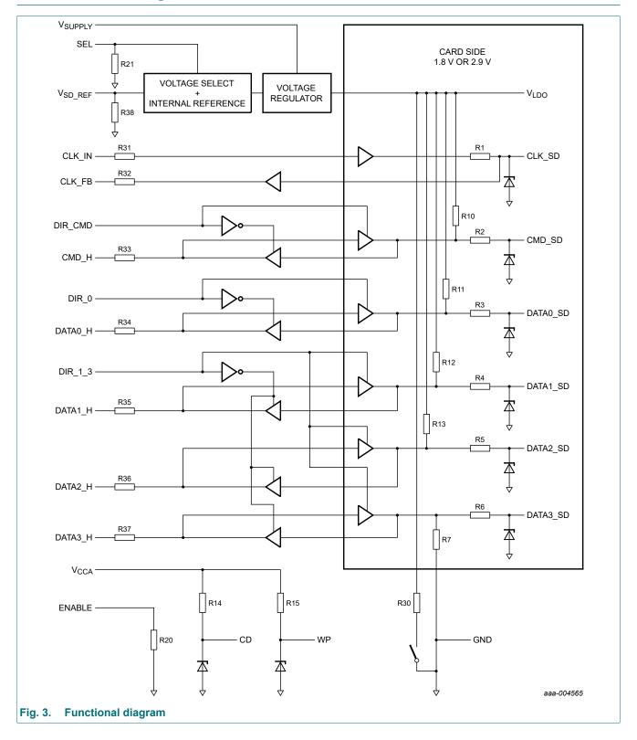
SD 3.0-compliant memory card integrated dual level translator with EMI filter and ESD protection
