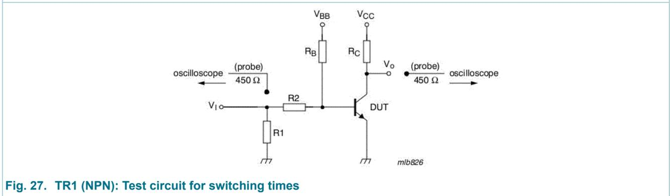
Fig. 27. TR1 (NPN): Test circuit for switching times
