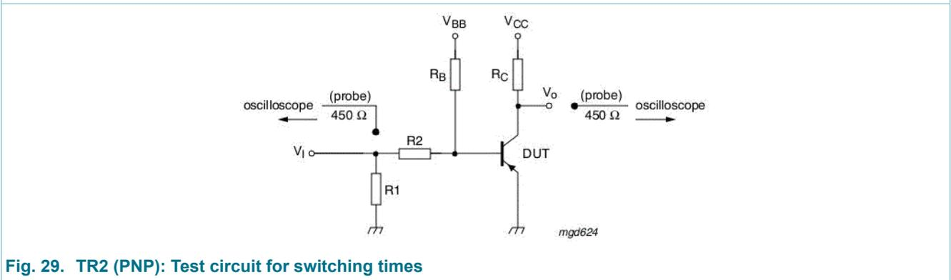
Fig. 29. TR2 (PNP): Test circuit for switching times
