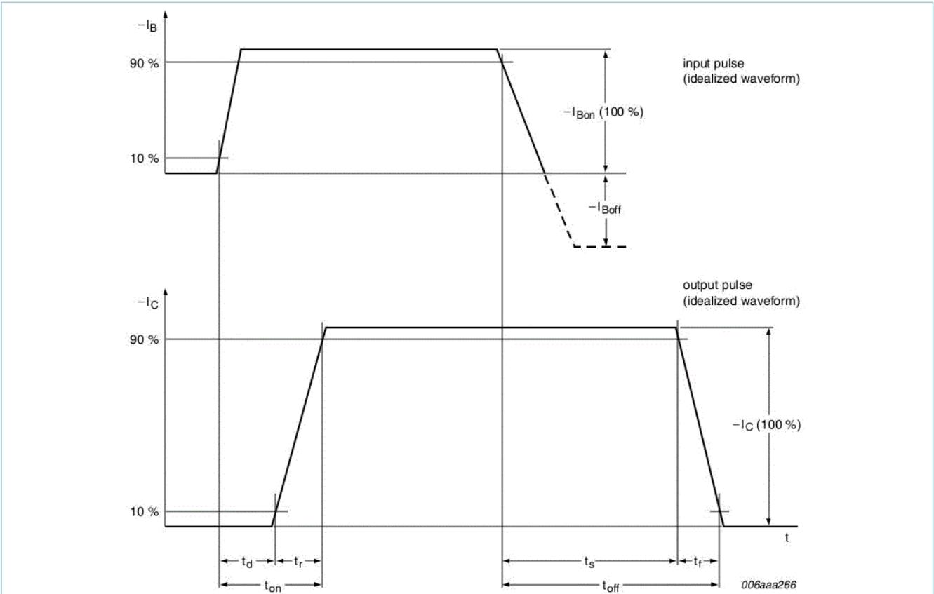
Fig. 28. TR2 (PNP): BISS transistor switching time definition
