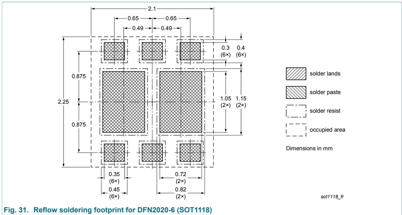
Fig. 31. Reflow soldering footprint for DFN2020-6 (SOT1118)
