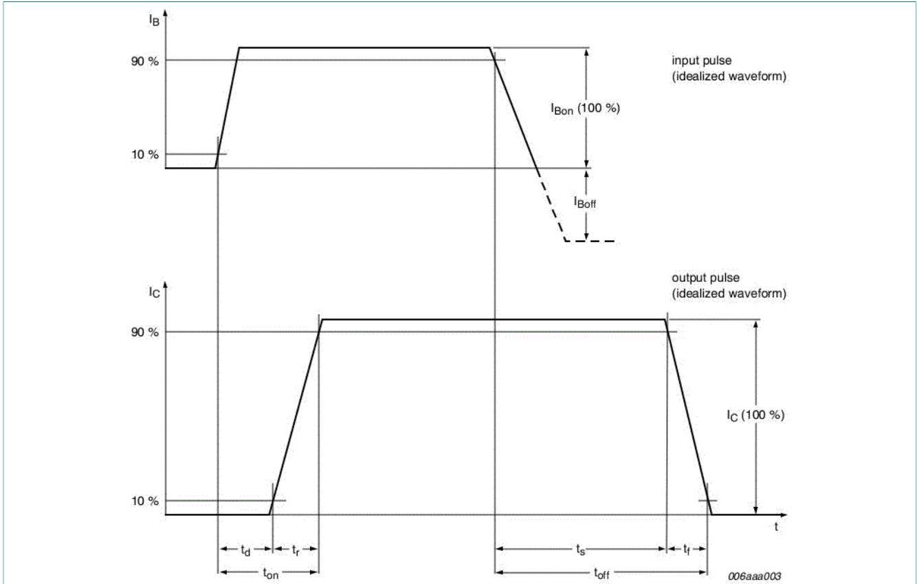
Fig. 26. TR1 (NPN): BISS transistor switching time definition
