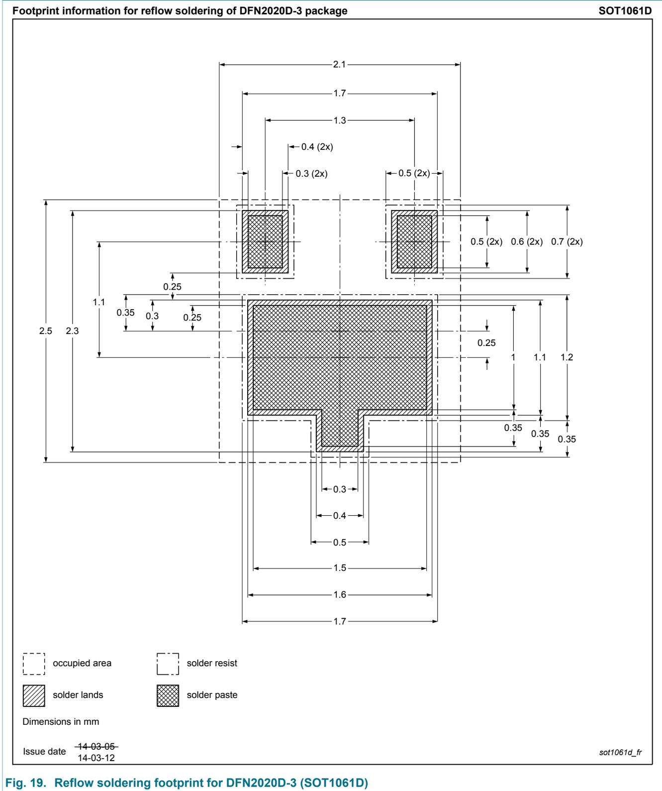
Fig. 19. Reflow soldering footprint for DFN2020D-3 (SOT1061D)
