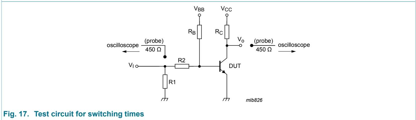
Fig. 17. Test circuit for switching times
