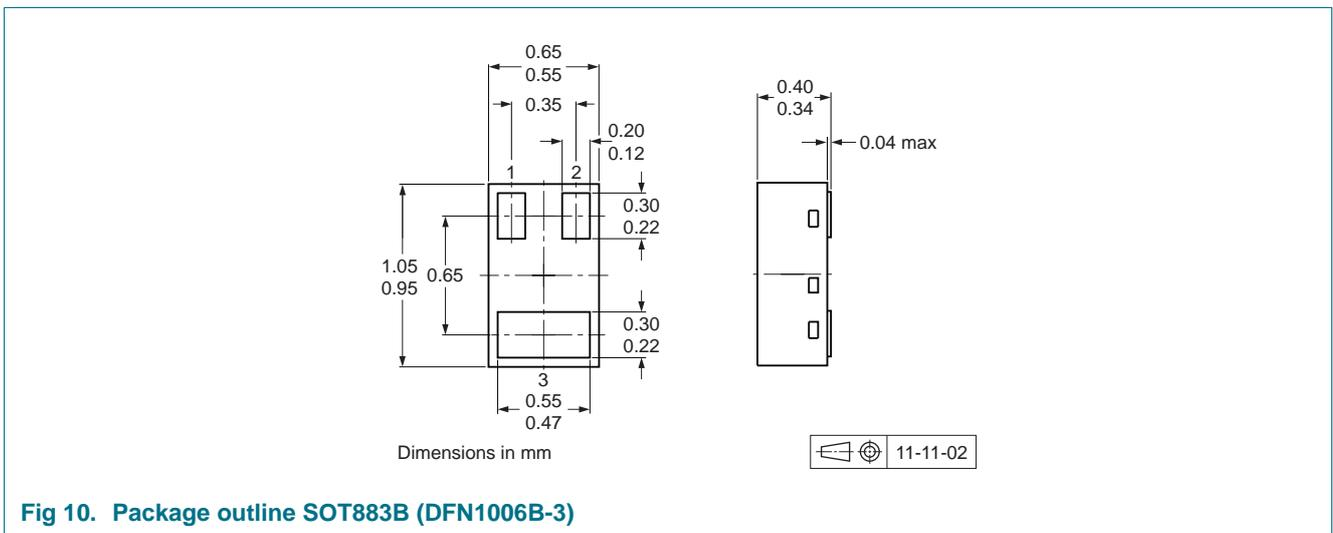
**Fig 10. Package outline SOT883B (DFN1006B-3)**
