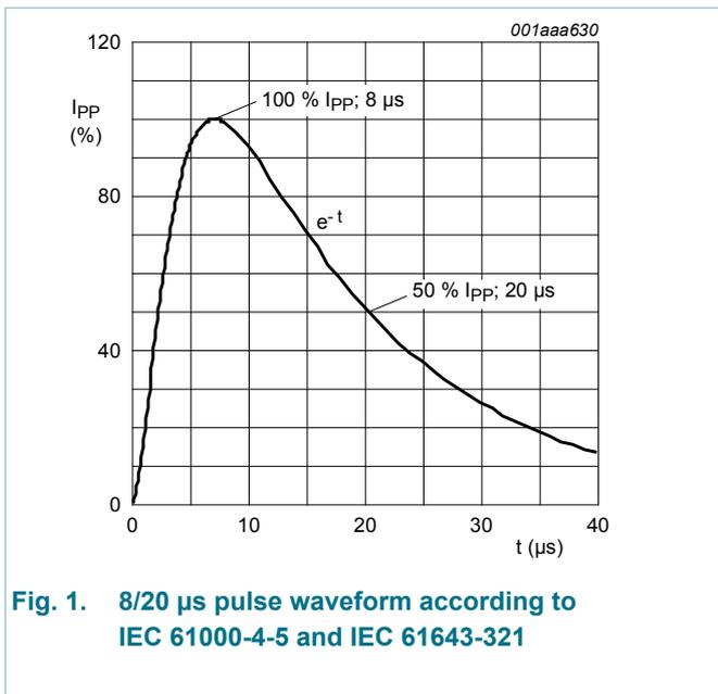
**Fig. 1. 8/20  $\mu s$  pulse waveform according to IEC 61000-4-5 and IEC 61643-321**
