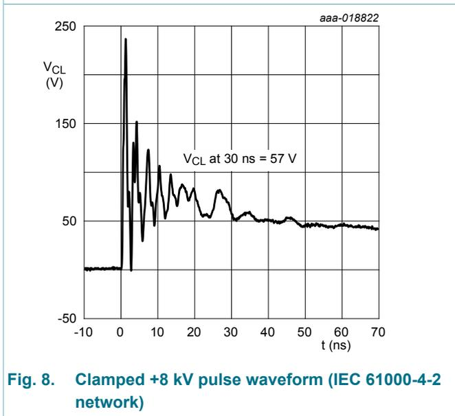
Fig. 8. Clamped +8 kV pulse waveform (IEC 61000-4-2 network)
