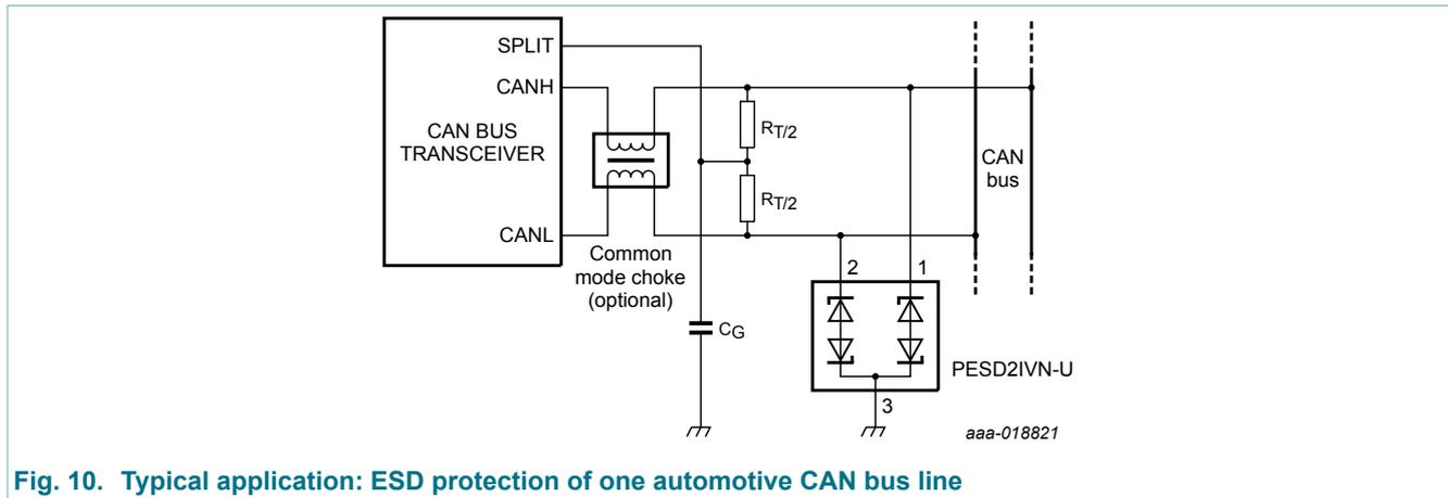
Fig. 10. Typical application: ESD protection of one automotive CAN bus line
