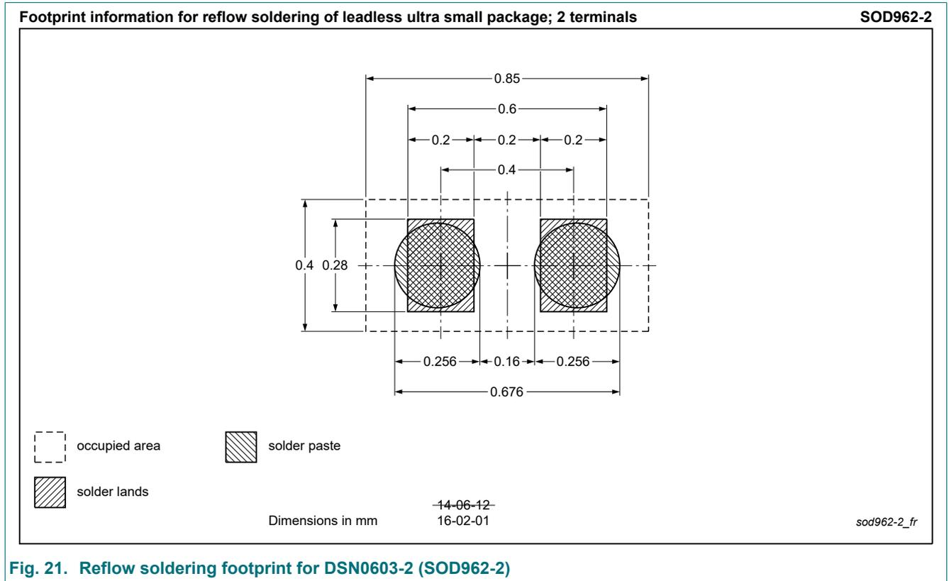
Fig. 21. Reflow soldering footprint for DSN0603-2 (SOD962-2)
