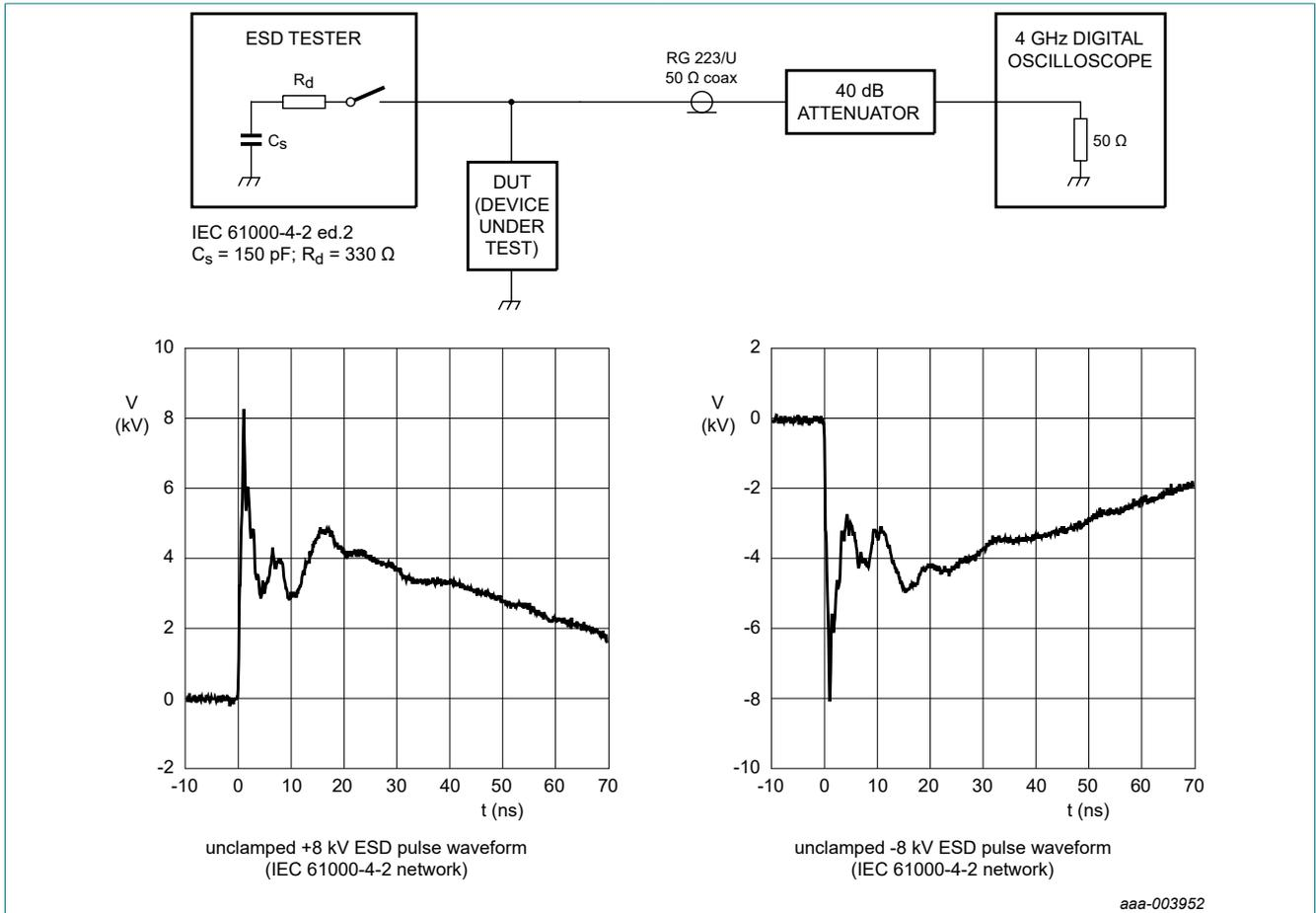
Fig. 7. ESD clamping test setup and waveforms
