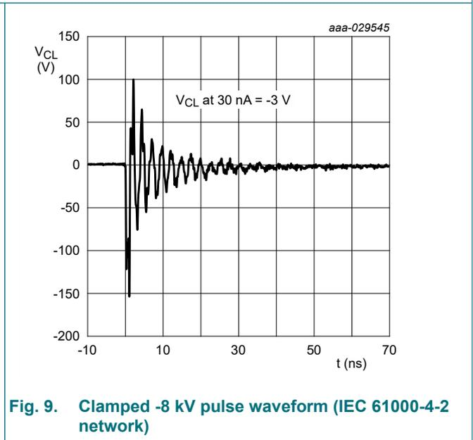
Fig. 9. Clamped -8 kV pulse waveform (IEC 61000-4-2 network)
