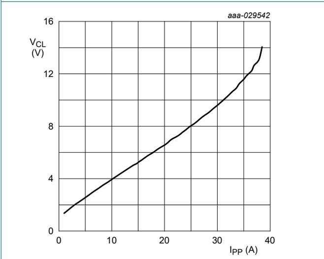
**Fig. 5. Positive clamping voltage (8/20 μs pulse); typical values**
