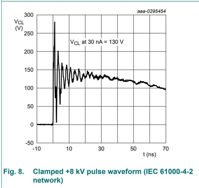
Fig. 8. Clamped +8 kV pulse waveform (IEC 61000-4-2 network)
