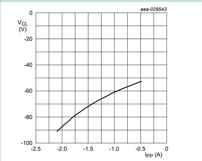
**Fig. 6. Negative clamping voltage (8/20 μs pulse); typical values**
