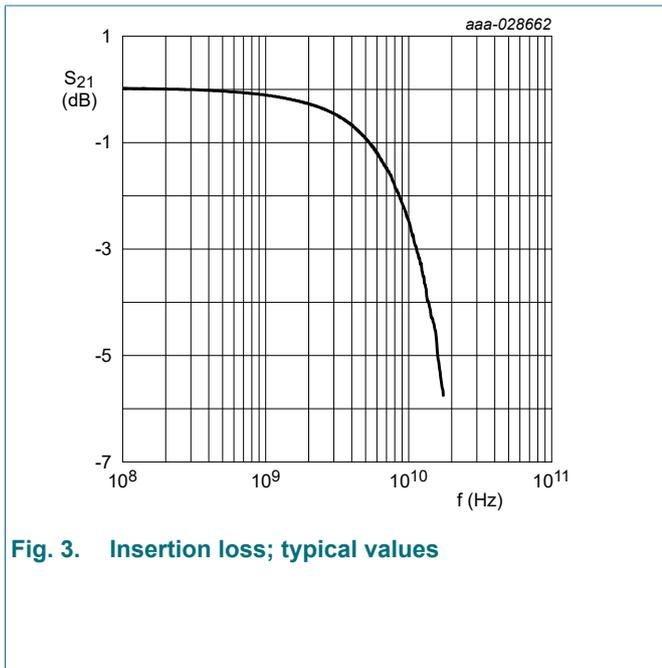
**Fig. 3. Insertion loss; typical values**
