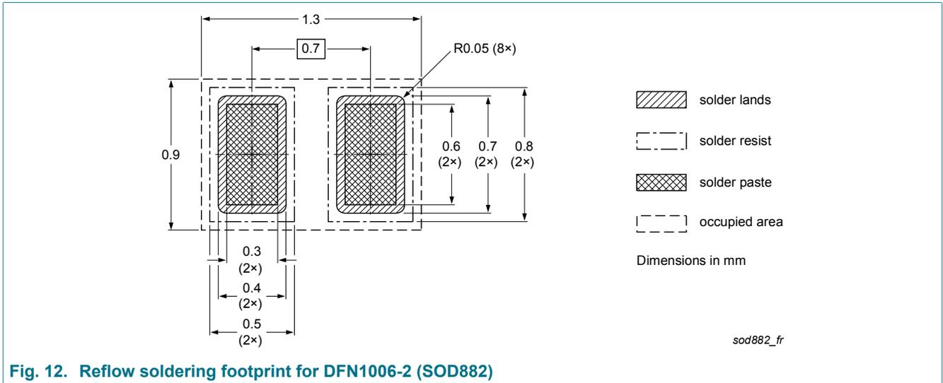
Fig. 12. Reflow soldering footprint for DFN1006-2 (SOD882)
