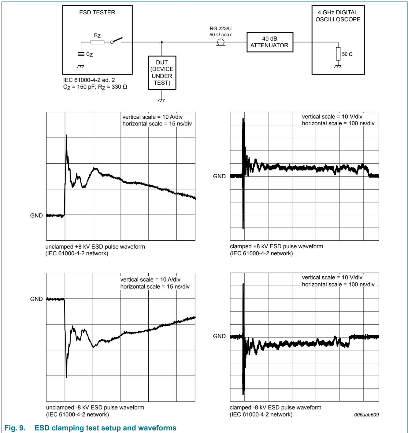
Fig. 9. ESD clamping test setup and waveforms
