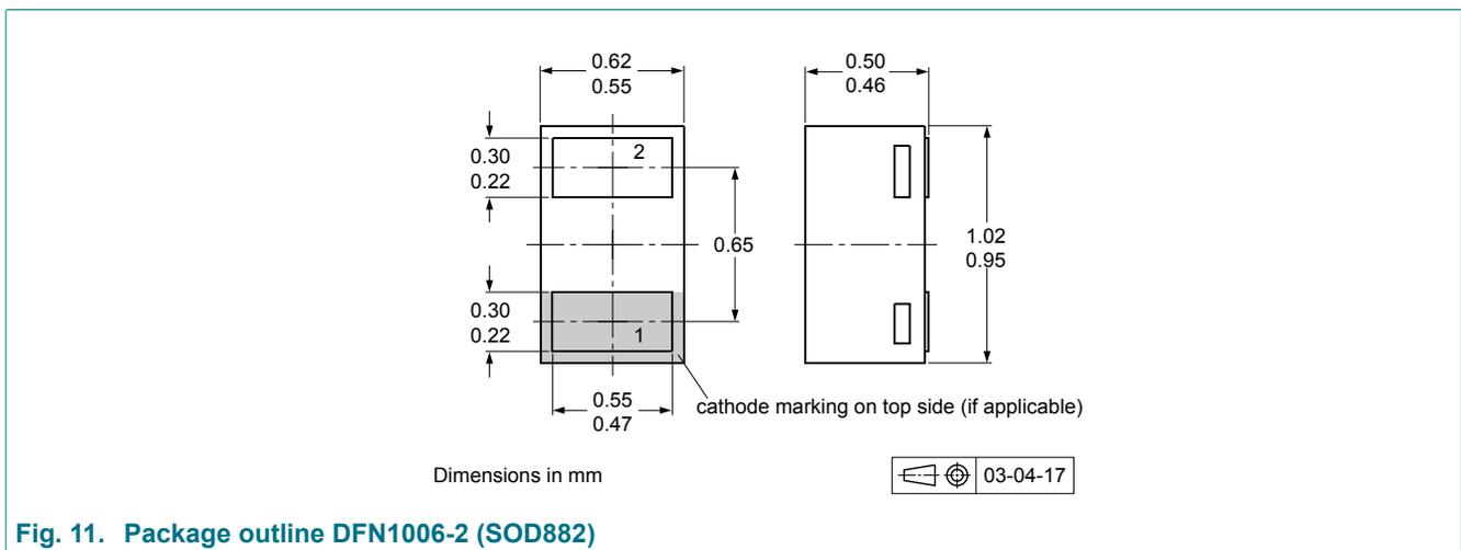
Fig. 11. Package outline DFN1006-2 (SOD882)
