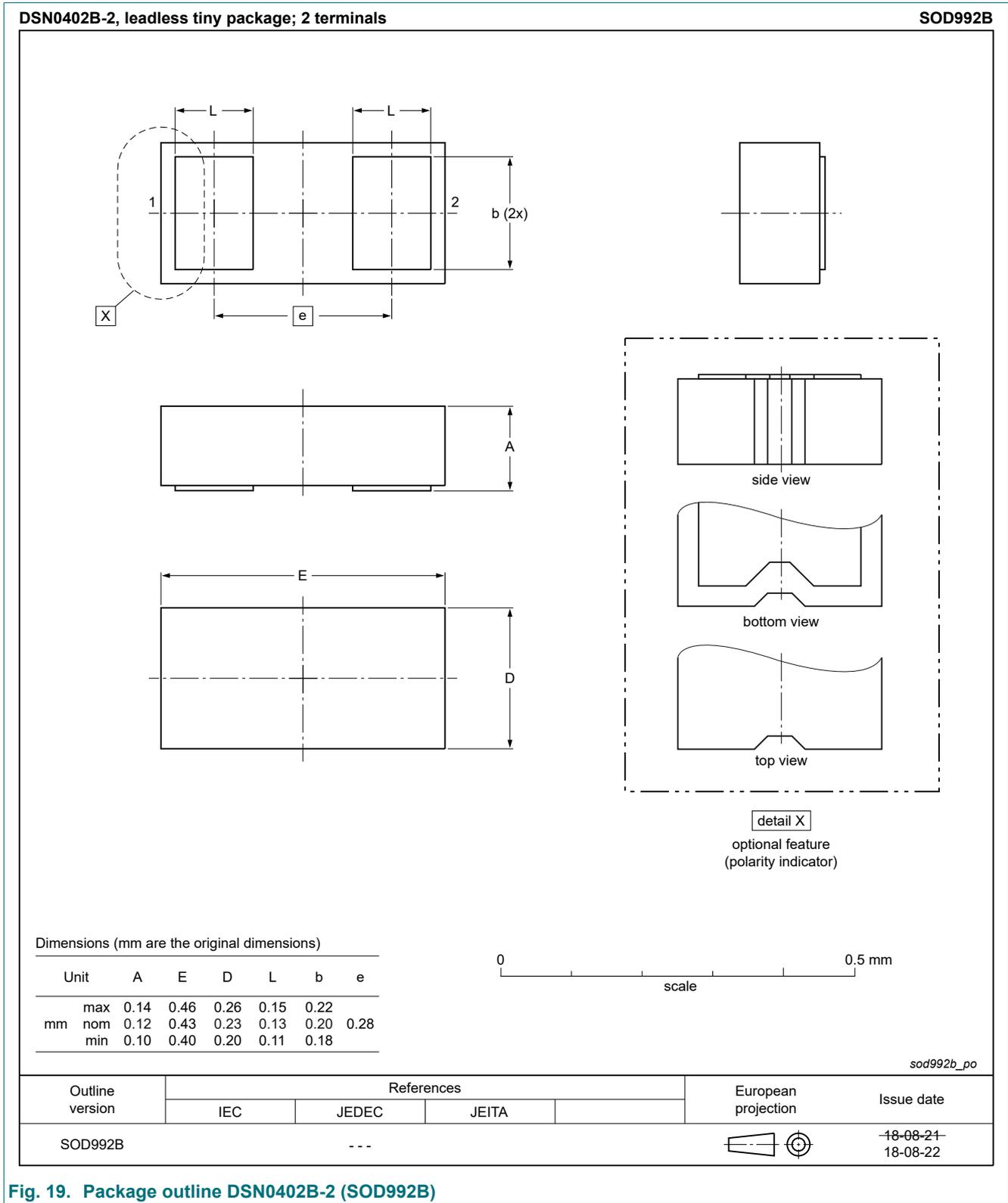
**Fig. 19. Package outline DSN0402B-2 (SOD992B)**
