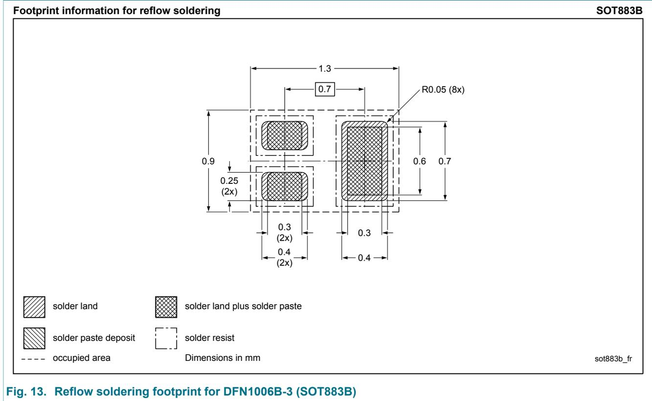
Fig. 13. Reflow soldering footprint for DFN1006B-3 (SOT883B)
