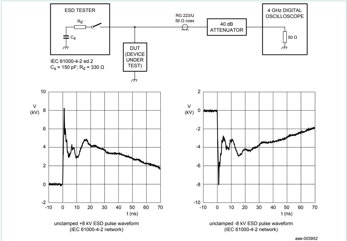
Fig. 8. ESD clamping test setup and waveforms
