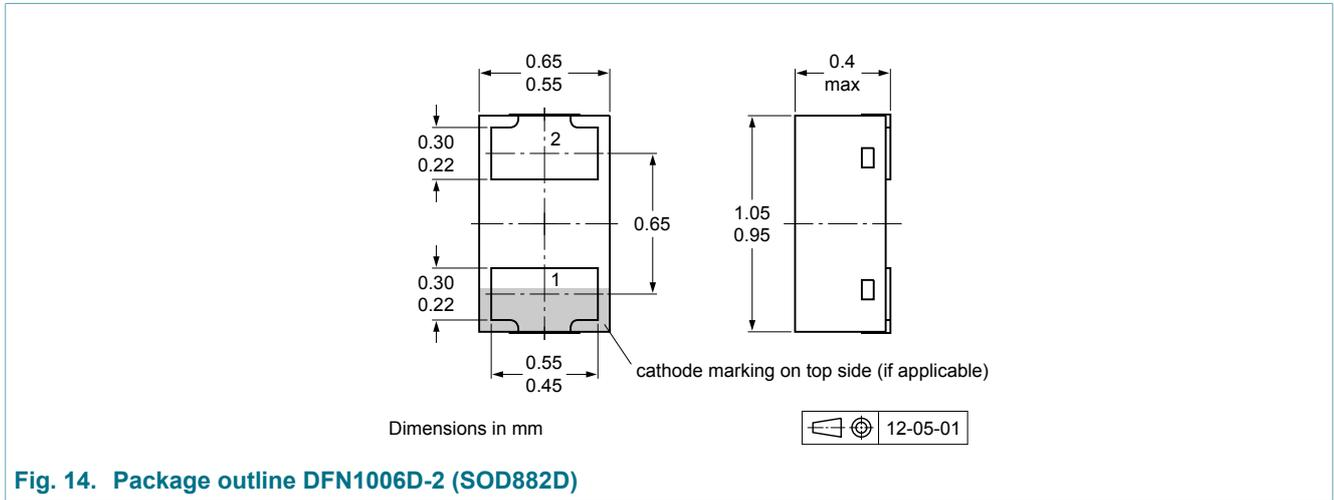
Fig. 14. Package outline DFN1006D-2 (SOD882D)
