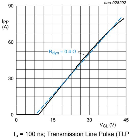
Fig. 6. Positive clamping voltage (TLP); typical values
