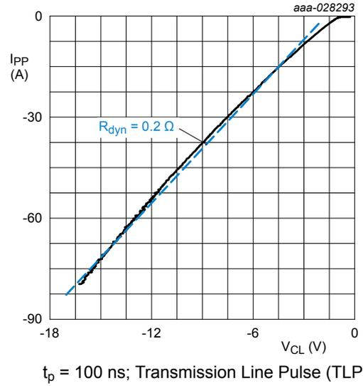
Fig. 7. Negative clamping voltage (TLP); typical values
