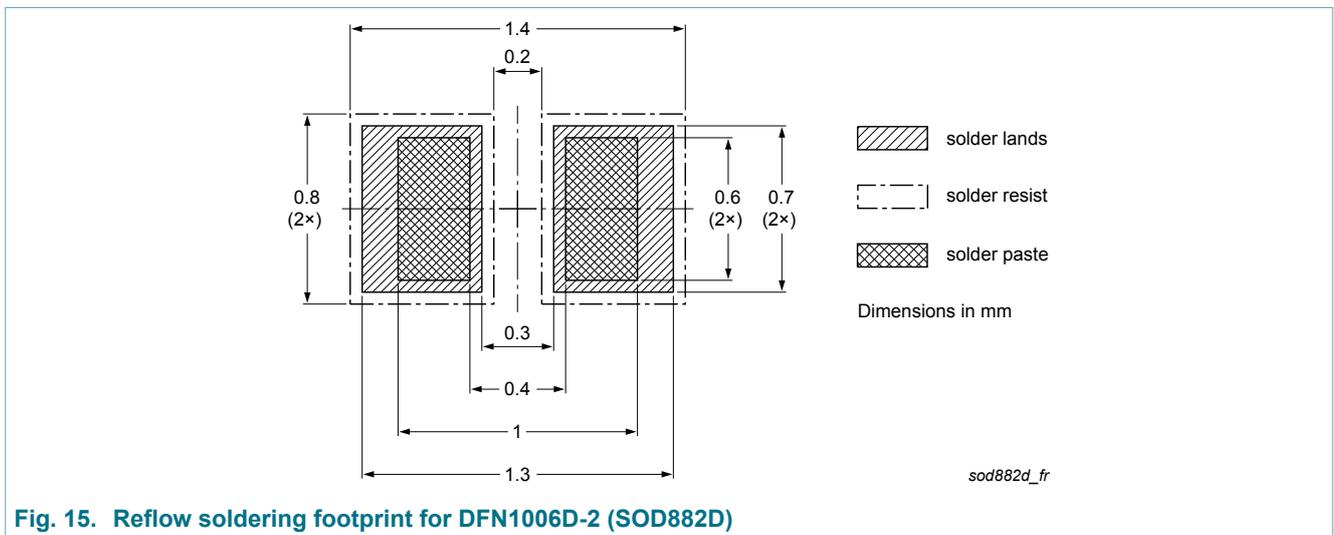
Fig. 15. Reflow soldering footprint for DFN1006D-2 (SOD882D)
