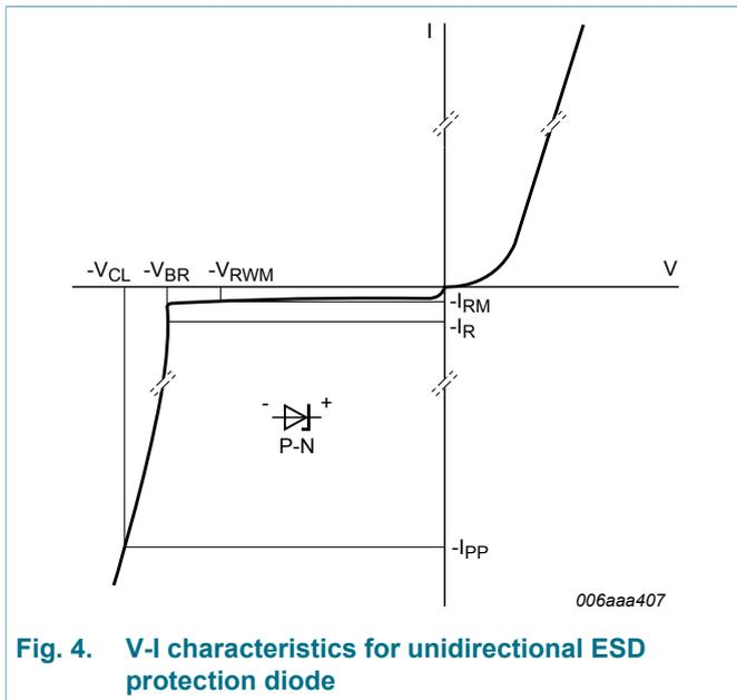
Fig. 4. V-I characteristics for unidirectional ESD protection diode
