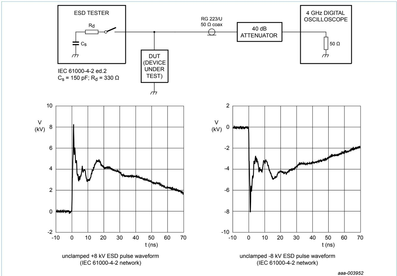
Fig. 10. ESD clamping test setup and waveforms
