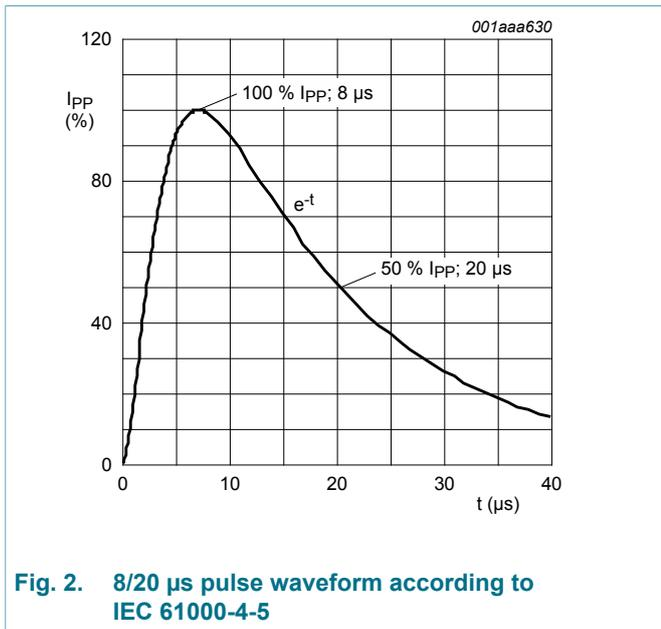
**Fig. 2. 8/20  $\mu s$  pulse waveform according to IEC 61000-4-5**
