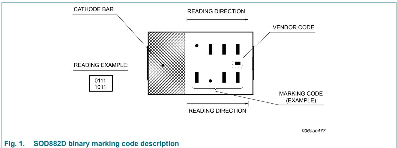
Fig. 1. SOD882D binary marking code description
