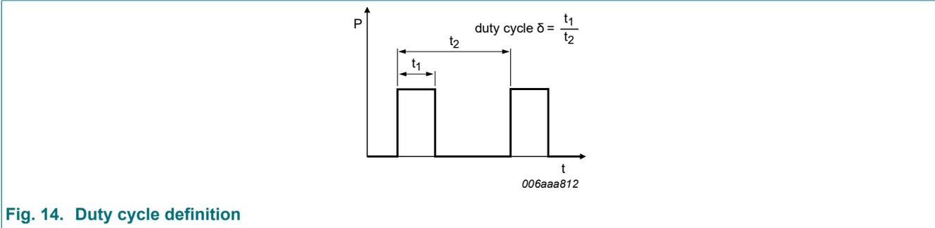
Fig. 14. Duty cycle definition
