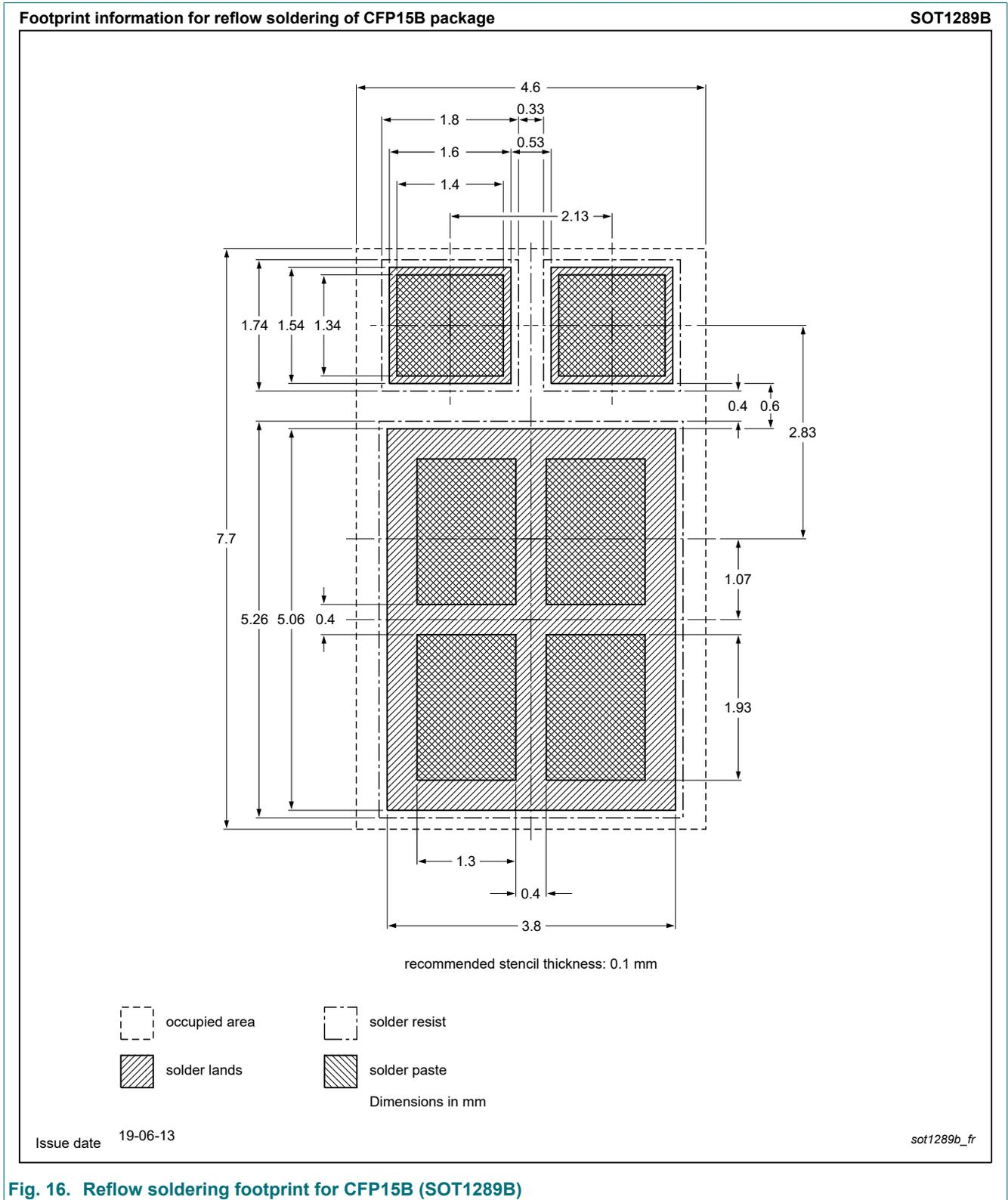
**Fig. 16. Reflow soldering footprint for CFP15B (SOT1289B)**
