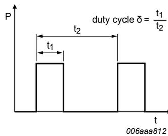
Fig. 13. Duty cycle definition
