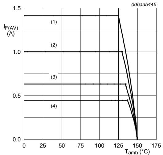
Ceramic PCB,  $\text{Al}_2\text{O}_3$ , standard footprint
