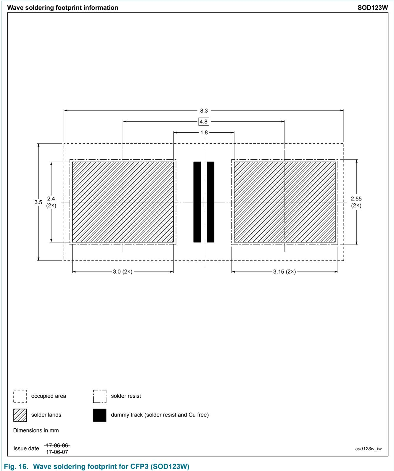
**Fig. 16. Wave soldering footprint for CFP3 (SOD123W)**
