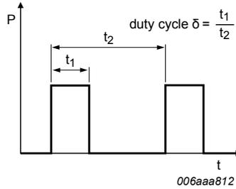
Fig. 14. Duty cycle definition
