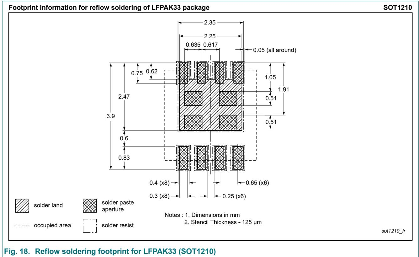
**Fig. 18. Reflow soldering footprint for LPAK33 (SOT1210)**
