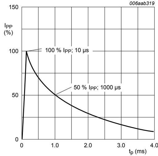
Fig. 3. 10/1000 μs pulse waveform according to IEC 61643-321
