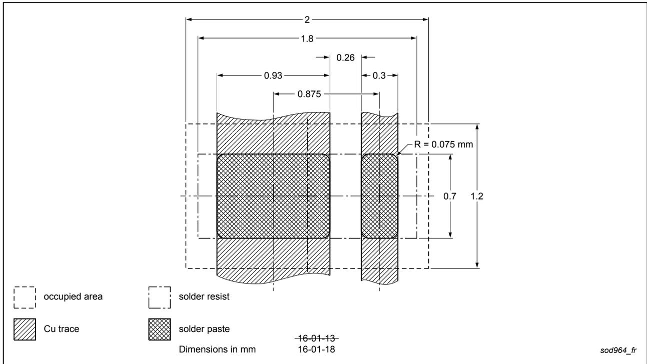
Fig. 17. Reflow soldering footprint for DSN1608-2 (SOD964)
