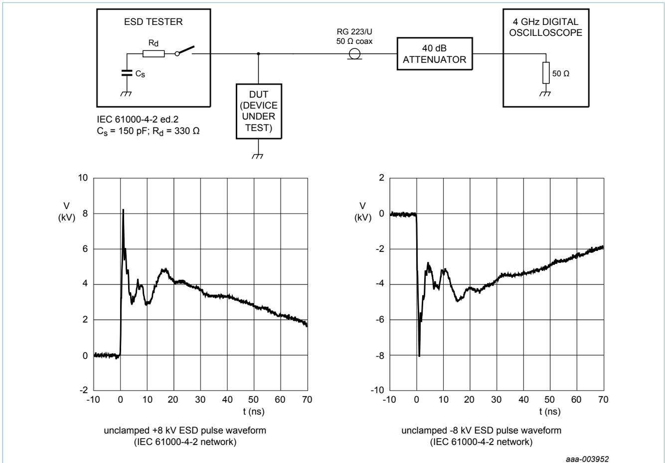
Fig. 12. ESD clamping test setup and waveforms
