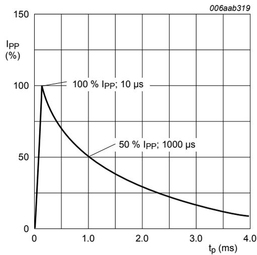
Fig. 3. 10/1000  $\mu$ s pulse waveform according to IEC 61643-321
