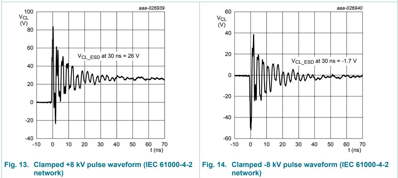
Fig. 13. Clamped +8 kV pulse waveform (IEC 61000-4-2 network)
