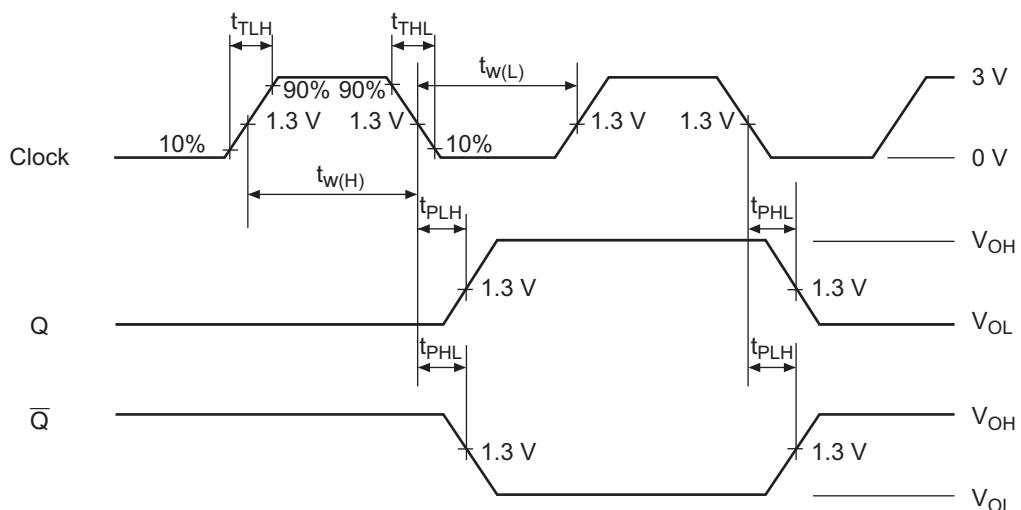
Note: Clock input pulse;  $t_{TLH} \leq 15$  ns,  $t_{THL} \leq 6$  ns, PRR = 1 MHz, duty cycle = 50% and for fmax.,  $t_{TLH} = t_{THL} \leq 2.5$  ns
