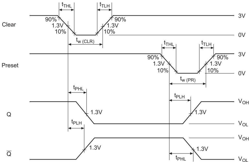
Note: Clear and preset input pulse;  $t_{TLH} \leq 15$  ns,  $t_{THL} \leq 6$  ns, PRR = 1 MHz,
