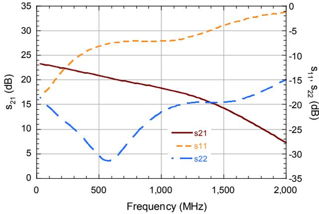
Performance vs. Frequency at  $P_{OUT} = 37\text{ dBm}$
