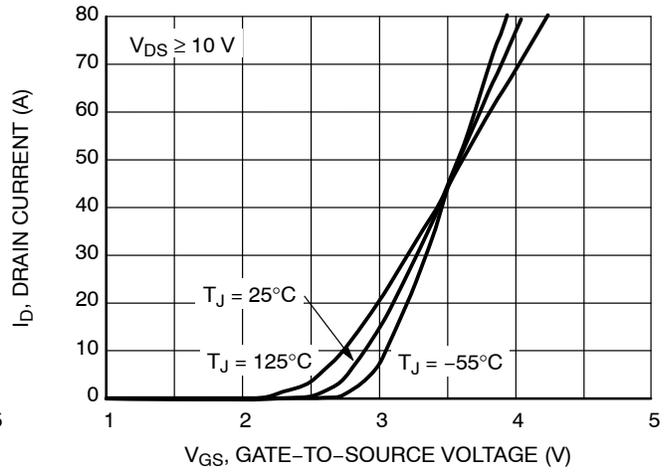
Figure 2. Transfer Characteristics
