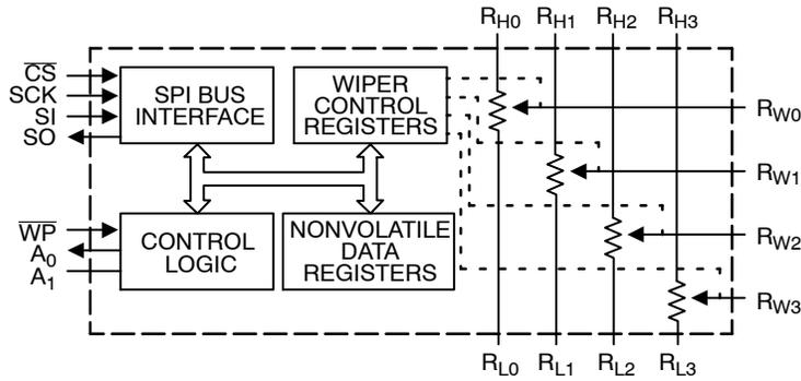
Figure 1. Functional Diagram
