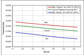
FIGURE 36-29: LFINTOSC Frequency, PIC16LF18325/18345 Only
