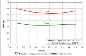
FIGURE 36-91: FVR Stabilization Period, PIC16LF18325/18345 Only
