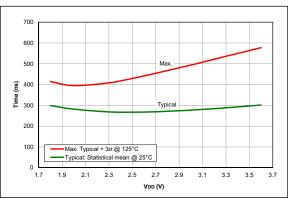
FIGURE 36-88: Comparator Response Time Rising edge, PIC16LF18325/18345 Only
