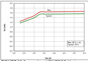
FIGURE 36-8: IDD, HFINTOSC Mode, Fosc = 16 MHz, PIC16F18325/18345 Only
