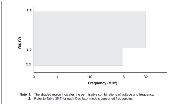
FIGURE 35-2: VOLTAGE FREQUENCY GRAPH, -40°C  $\leq$  Ta  $\leq$  +125°C, PIC16LF18325/18345 ONLY
