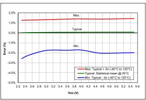
FIGURE 36-27: HFINTOSC Typical Frequency Error, PIC16F18325/18345 Only
