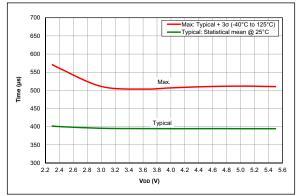
FIGURE 36-113: Wake From Sleep, VREGPM = 1, LFINTOSC, PIC16F18325/18345 Only
