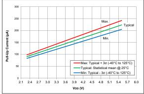
FIGURE 36-31: Weak Pull-Up Current, PIC16F18325/18345 Only
