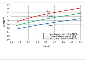
FIGURE 36-99: TTL Trip Thresholds, All devices
