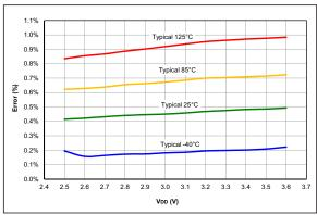
**FIGURE 36-92:** Typical FVR Voltage (1x), PIC16LF18325/18345 Only
