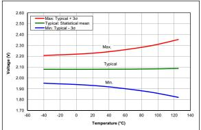
FIGURE 36-45: LPBOR Reset Voltage, PIC16LF18325/18345 only
