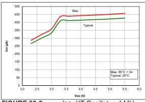
**FIGURE 36-2:** IDD, XT Oscillator, 4 MHz, PIC16F18325/18345 Only
