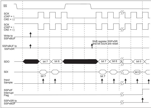
FIGURE 30-9: SPI MODE WAVEFORM (SLAVE MODE WITH CKE = 0) SS Optional SCK (CKP = 0 CKE = 0) SCK (CKP = 1 CKE = 0) Write to **SSPxBUF** Valid bit 4 SDO bit 7 bit 6 bit 5 bit 3 bit 2 bit 1 bit 0 SDI bit 7 Input Sample SSPxIF Interrupt Flag SSPxSR to SSPxBUF -
