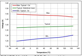
FIGURE 36-105: POR Release Voltage, All devices
