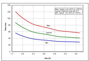
FIGURE 36-84: Comparator Response Time Over Voltage, Normal Power Mode (CxSP = 1), VDD = 5.5V, Typical Measured Values PIC16LF18325/18345 Only
