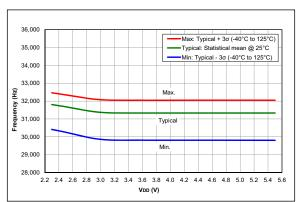
FIGURE 36-30: LFINTOSC Frequency, PIC16F18325/18345 Only
