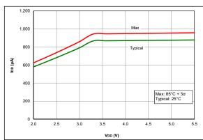
FIGURE 36-10: IDD, HFINTOSC IDLE Mode, Fosc = 16 MHz, PIC16F18325/18345 Only
