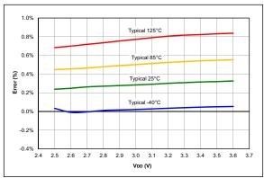
**FIGURE 36-94:** FVR Voltage Error (2x), PIC16LF18325/18345 Only
