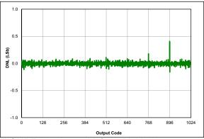
FIGURE 36-51: ADC 10-Bit Mode. Single-Ended DNL, VDD = 3.0V, VREF = 3.0V,  $TAD = 8 \mu s$ , 25°C, All devices
