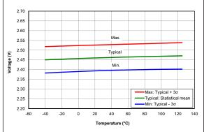
FIGURE 36-43: Brown-out Reset Voltage, Trip Point, (BORV = 1), PIC16F18325/18345 Only
