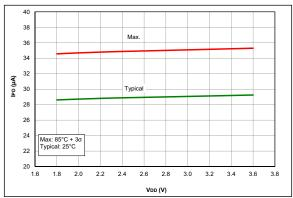
FIGURE 36-22: IPD, Comparator, PIC16LF18325/18345 Only
