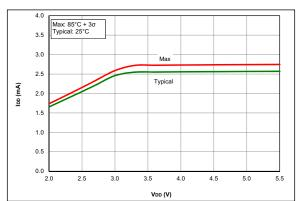
FIGURE 36-6: IDD, HFINTOSC Mode, Fosc = 32 MHz, PIC16F18325/18345 Only
