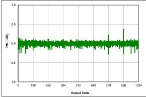
FIGURE 36-49: ADC 10-Bit Mode. Single-Ended DNL, VDD = 3.0V, VREF = 3.0V,  $TAD = 1 \mu s$ , 25°C, All devices
