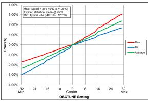
FIGURE 36-104: OSCTUNE Center Frequency, PIC16LF18325/18345 Only
