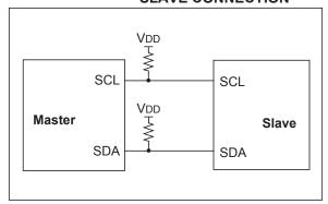
On the last byte of data communicated, the master device may end the transmission by sending a Stop bit. If the master device is in Receive mode, it sends a  $\overline{\text{NACK}}$  in place of the last  $\overline{\text{ACK}}$  bit. A Stop bit is indicated by a low-to-high transition of the SDA line while the SCL line is held high.
