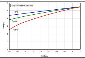
**FIGURE 36-33:** VOH vs. IOH Over Temperature, VDD = 5.5V, PIC16F18325/18345 Only
