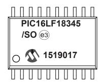
20-Lead SSOP (5.30 mm)
