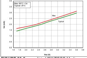
FIGURE 36-5: IDD, HFINTOSC Mode, Fosc = 32 MHz, PIC16LF18325/18345 Only
