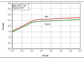
**FIGURE 36-4:** IDD, HS Oscillator, 32 MHz, PIC16F18325/18345 Only
