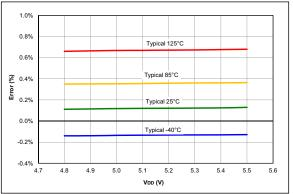
**FIGURE 36-96:** FVR Voltage Error (4x), PIC16F18325/18345 Only
