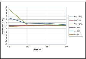
FIGURE 36-63: ADC 10-Bit Mode, Single-Ended Gain Error, VDD = 3.0V, TAD = 4 µs, All devices
