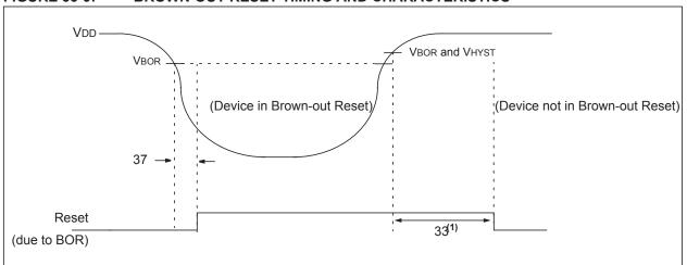
**Note 1:** 64 ms delay only if  $\overline{\text{PWRTE}}$  bit in the Configuration Word register is programmed to '0'. 2 ms delay if  $\overline{\text{PWRTE}} = 0$ .
