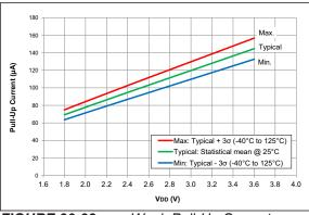
FIGURE 36-32: Weak Pull-Up Current, PIC16LF18325/18345 Only
