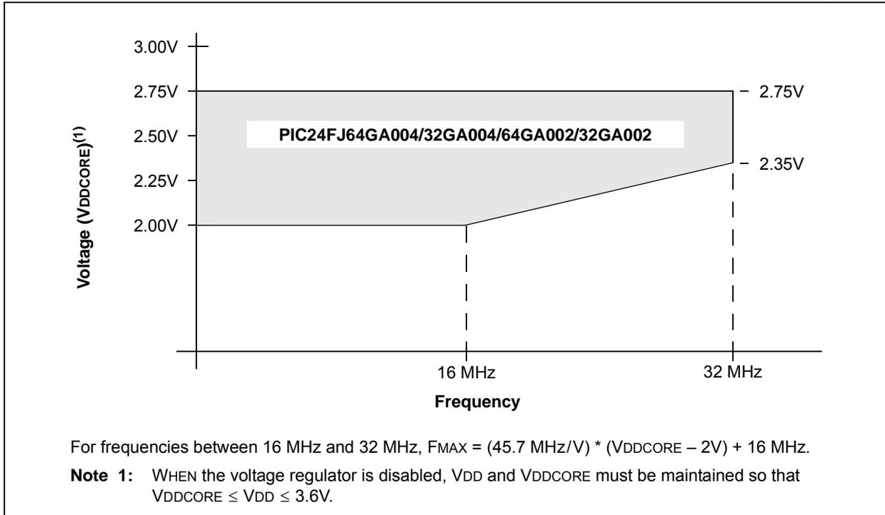
FIGURE 27-2: PIC24FJ64GA004 FAMILY VOLTAGE-FREQUENCY GRAPH (EXTENDED TEMPERATURE)
