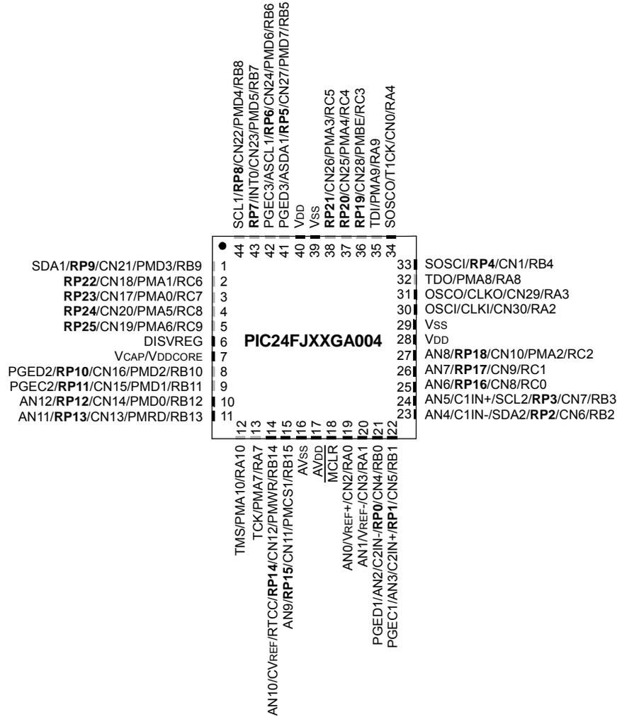
**Legend:** RP<sub>n</sub> represents remappable peripheral pins. Gray shading indicates 5.5V tolerant input pins.
