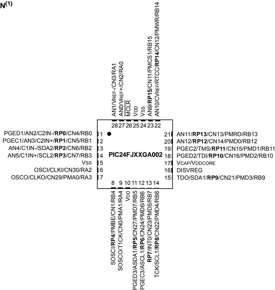
**Legend:** RPn represents remappable peripheral pins. Gray shading indicates 5.5V tolerant input pins.
