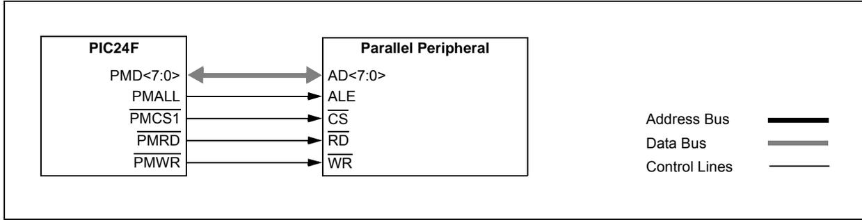
**FIGURE 18-10: PARALLEL EEPROM EXAMPLE (UP TO 11-BIT ADDRESS, 8-BIT DATA)**
