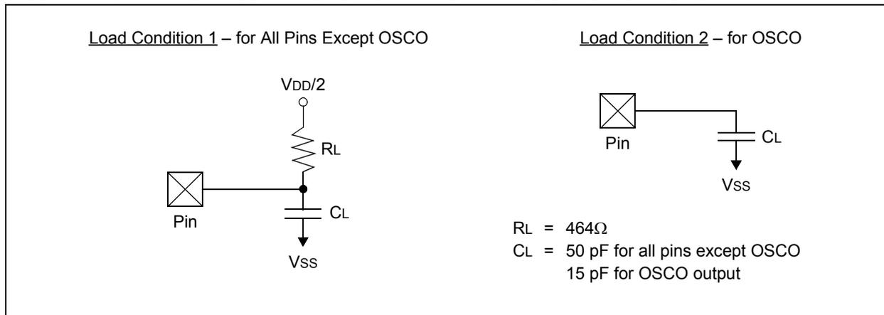
**TABLE 27-14: CAPACITIVE LOADING REQUIREMENTS ON OUTPUT PINS**
