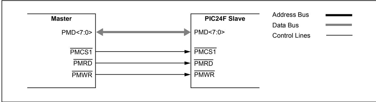
**FIGURE 18-3: ADDRESSABLE PARALLEL SLAVE PORT EXAMPLE**
