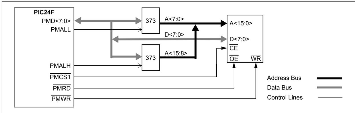
**FIGURE 18-8: EXAMPLE OF A PARTIALLY MULTIPLEXED ADDRESSING APPLICATION**
