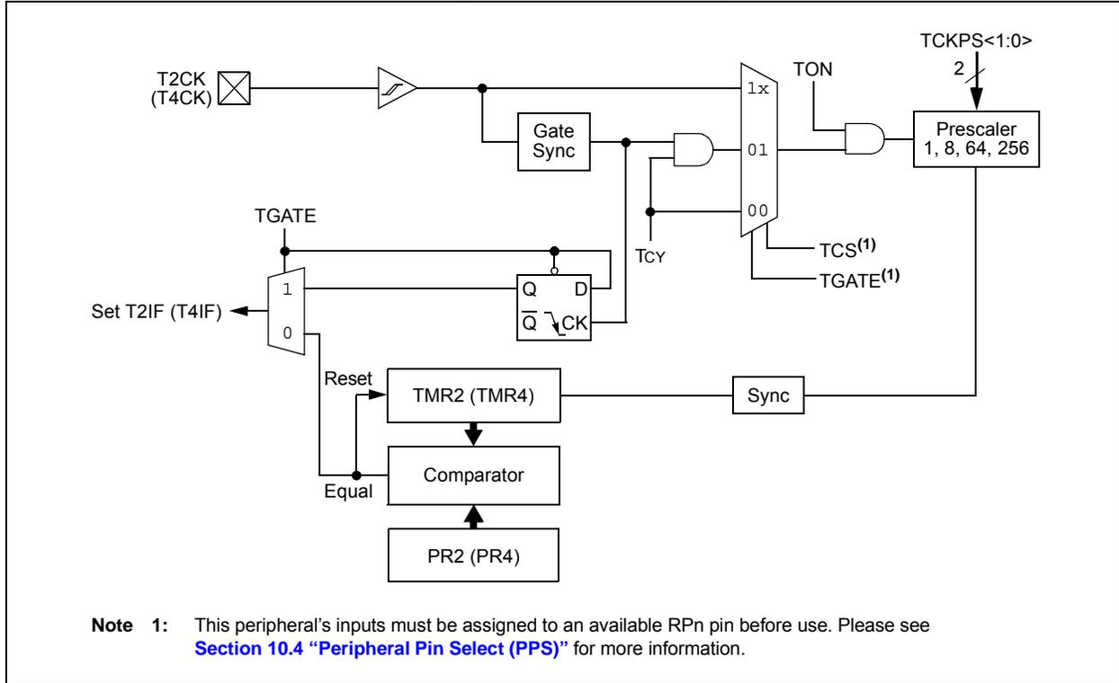
**FIGURE 12-3: TIMER3 AND TIMER5 (16-BIT SYNCHRONOUS) BLOCK DIAGRAM**
