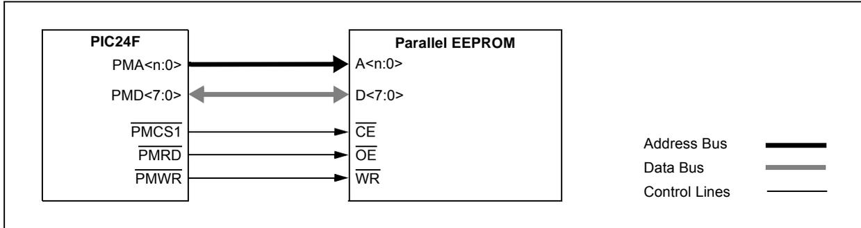
**FIGURE 18-11: PARALLEL EEPROM EXAMPLE (UP TO 11-BIT ADDRESS, 16-BIT DATA)**
