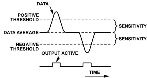
Figure 37. Threshold Sensitivity
