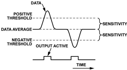
Figure 31. Threshold Sensitivity
