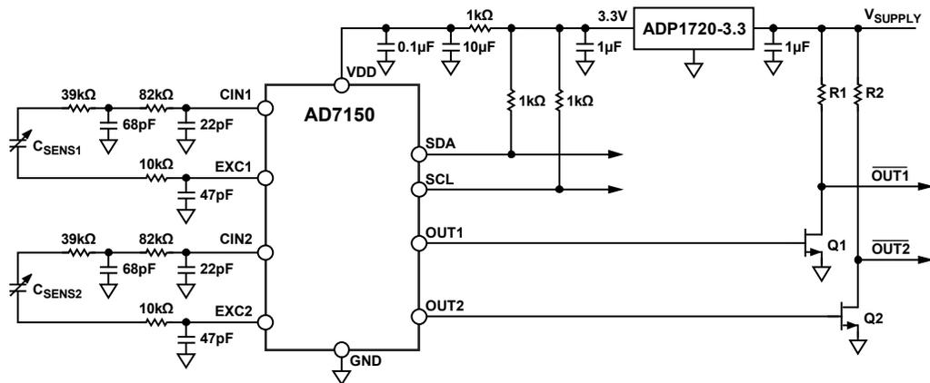
Figure 53. AD7150 Standalone Operation with EMC Protection
