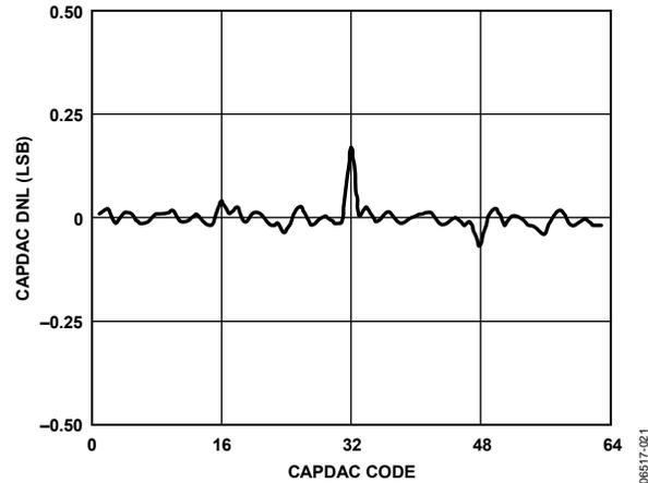
Figure 21. CAPDAC Differential Nonlinearity (DNL),  $V_{DD} = 3.3\text{ V}$
