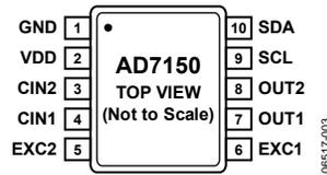
Figure 3. Pin Configuration
