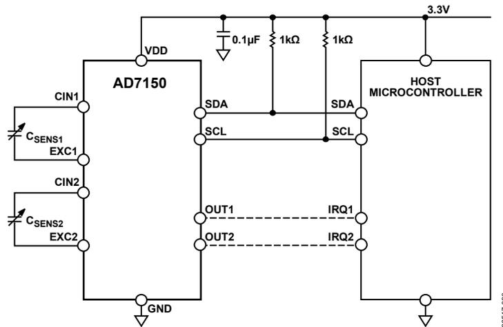
Figure 52. AD7150 Interfaced to a Host Microcontroller
