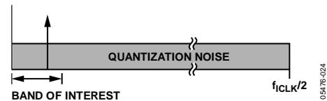
Figure 23.  $\Sigma$ - $\Delta$  ADC, Quantization Noise
