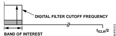
Figure 25.  $\Sigma$ - $\Delta$  ADC, Digital Filter Cutoff Frequency
