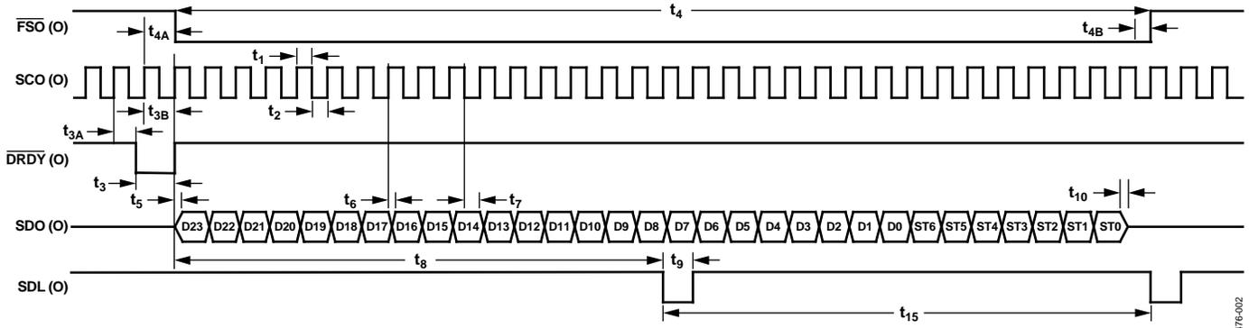
Figure 2. SPI® Interface Serial Read Timing Diagram
