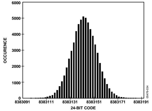
Figure 21. Low Power 24-Bit Histogram, 256x Decimation
