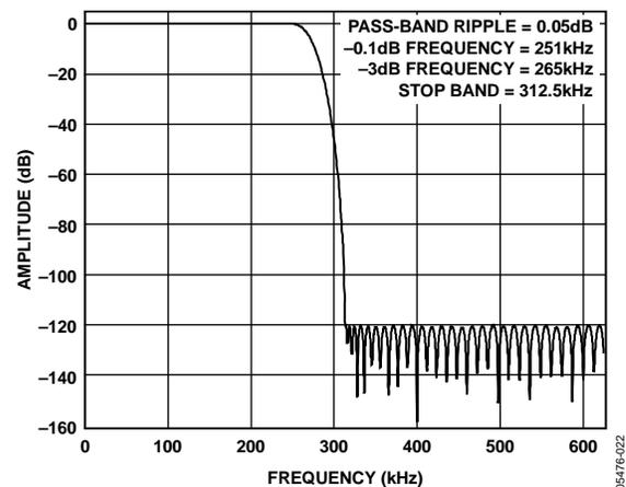
Figure 37. Default Filter Frequency Response (625 kHz ODR)
