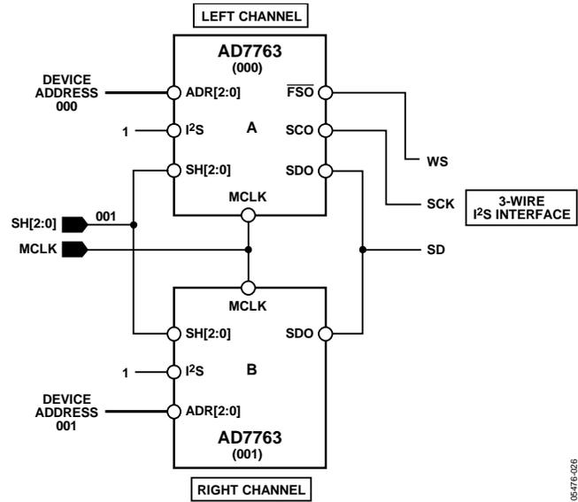
Figure 27. Two AD7763 Devices Operating Using the I<sup>2</sup>S Interface
