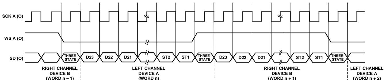
Figure 28. Timing Diagram for I<sup>2</sup>S Interface
