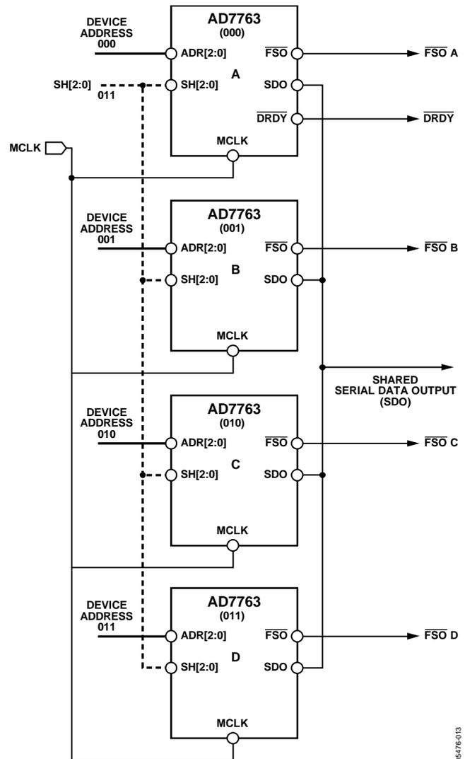
Figure 26. Four AD7763 Devices Sharing the Serial Bus
