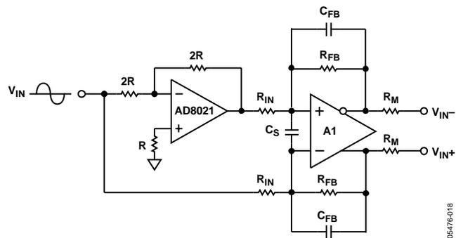
Figure 33. Single-Ended-to-Differential Conversion
