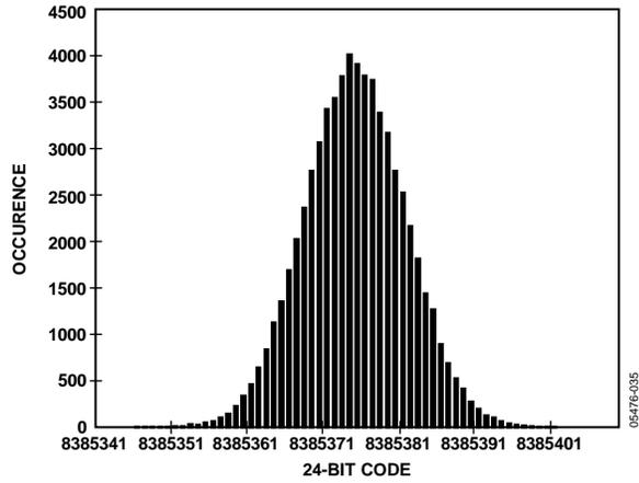
Figure 18. Normal Mode, 24-Bit Histogram, 256x Decimation
