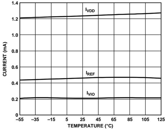
Figure 23. Operating Currents for Each ADC vs. Temperature
