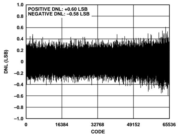
Figure 9. Differential Nonlinearity vs. Code,  $V_{REF} = 2.5\text{ V}$
