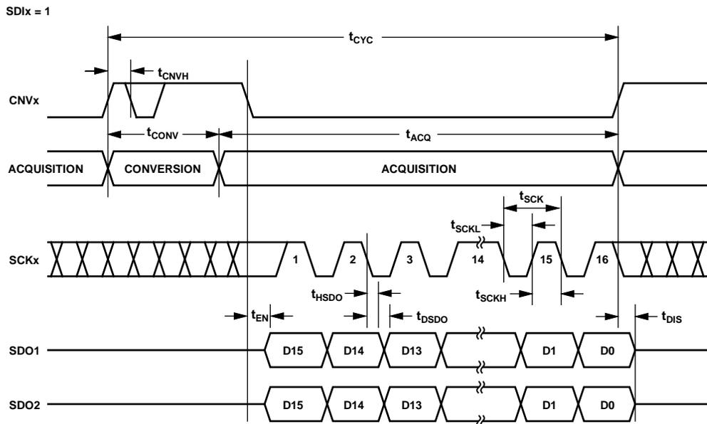
Figure 51. Potential Simultaneous Sampling Serial Interface Timing
