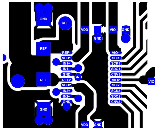
Figure 53. Example Layout of the [AD7902](#) (Top Layer)
