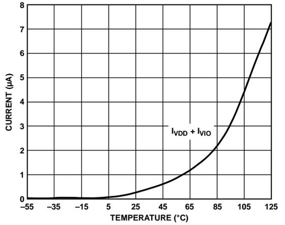
Figure 26. Power-Down Current for Each ADC vs. Temperature
