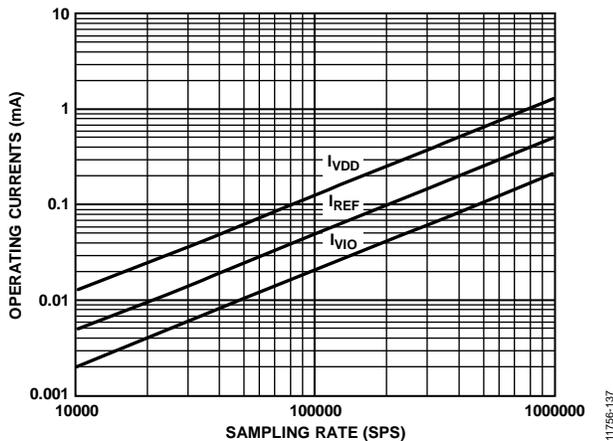
Figure 37. Operating Currents per ADC vs. Sampling Rate
