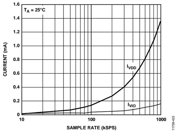
Figure 22. Operating Currents for Each ADC vs. Throughput
