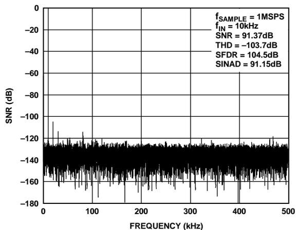
Figure 7. FFT Plot,  $V_{REF} = 5\text{ V}$
