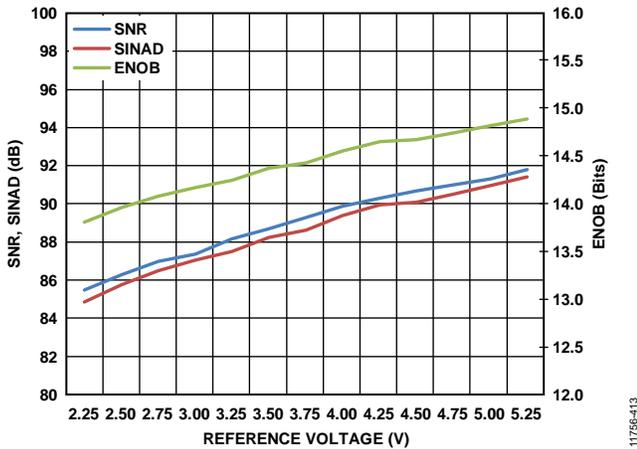
Figure 13. SNR, SINAD, and ENOB vs. Reference Voltage
