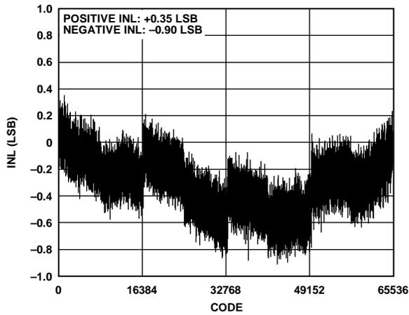
Figure 5. Integral Nonlinearity vs. Code,  $V_{REF} = 5\text{ V}$
