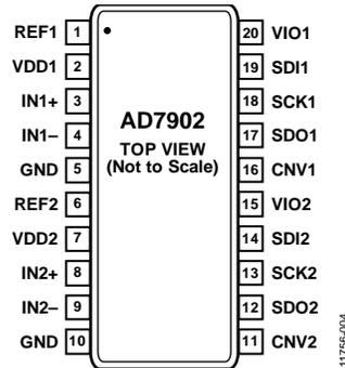
Figure 4. Pin Configuration
