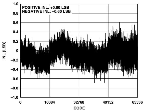
Figure 6. Integral Nonlinearity vs. Code,  $V_{REF} = 2.5\text{ V}$
