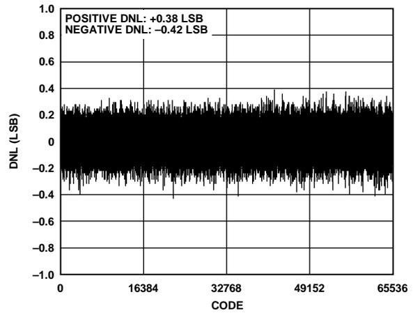
Figure 8. Differential Nonlinearity vs. Code,  $V_{REF} = 5\text{ V}$
