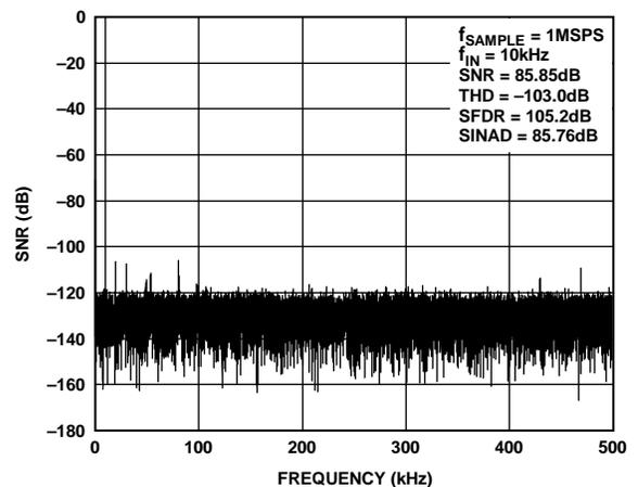
Figure 10. FFT Plot,  $V_{REF} = 2.5\text{ V}$
