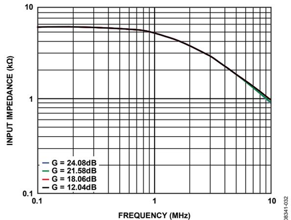
Figure 13. Input Impedance  $R_{IN}$  vs. Frequency, Underterminated
