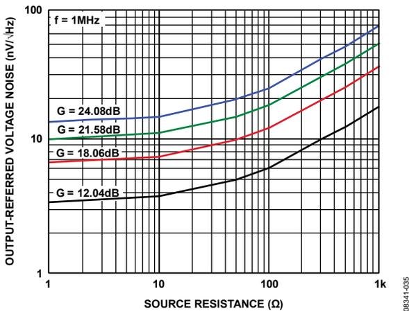
Figure 17. Output-Referred Voltage Noise vs. Source Resistance ( $R_s$ )
