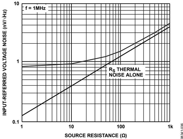
Figure 16. Input-Referred Voltage Noise vs. Source Resistance ( $R_s$ )
