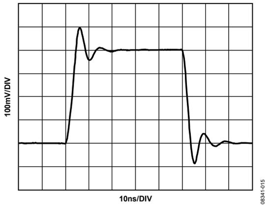
Figure 40. Small Signal Transient Response,  $G = 12.04 \text{ dB}$
