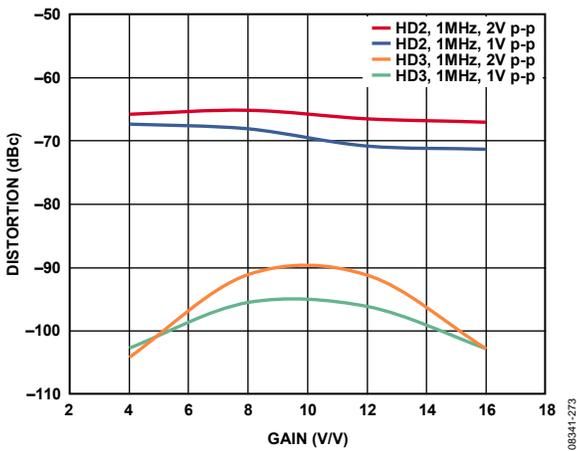
Figure 35. Harmonic Distortion at 1 MHz vs. Gain
