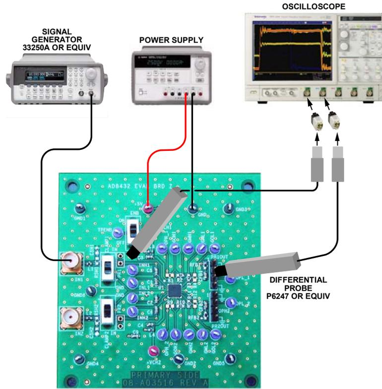
Figure 79. Bench Setup for Testing the AD8432-EVALZ
