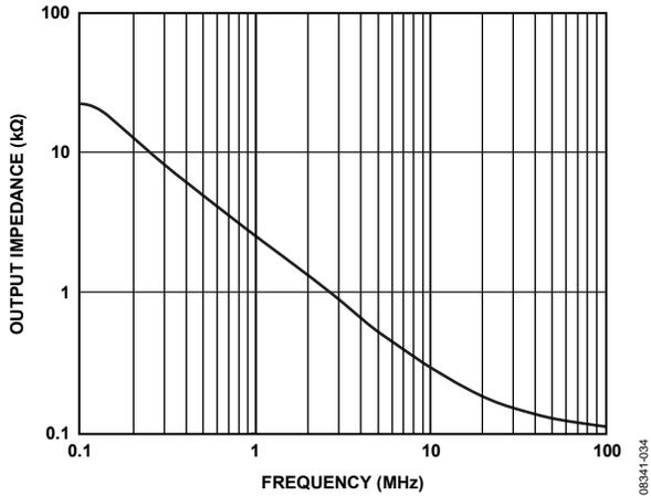
Figure 15. Output Impedance vs. Frequency in Disable Mode
