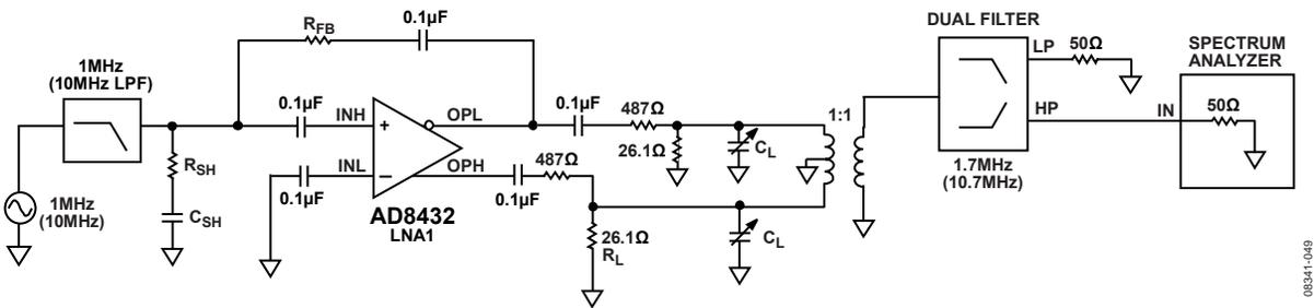
Figure 58. Harmonic Distortion vs. Capacitive Load ( $C_L$ ) Measurements
