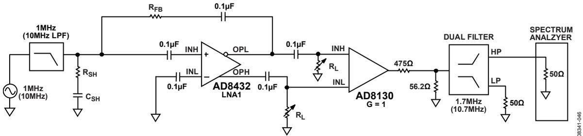
Figure 57. Harmonic Distortion vs. Resistive Load ( $R_L$ ) Measurements
