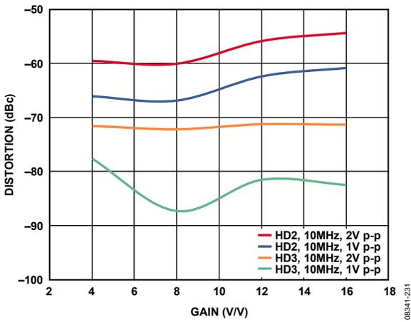
Figure 34. Harmonic Distortion at 10 MHz vs. Gain
