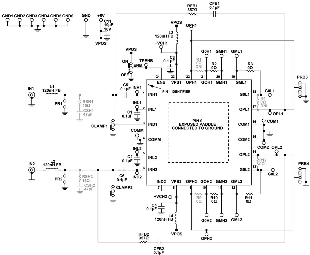
Figure 80. AD8436-EVALZ Schematic
