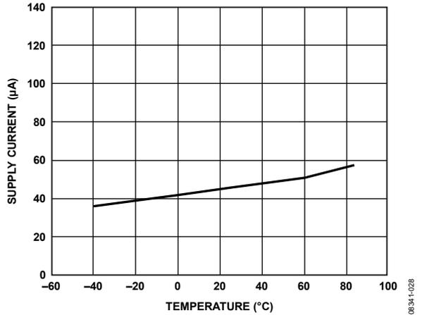
Figure 54. Supply Current vs. Temperature in Disable Mode
