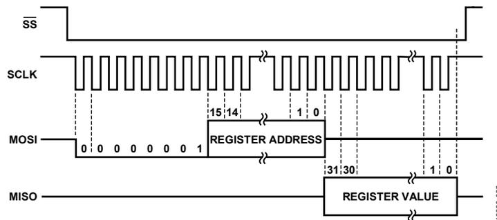
Figure 45. SPI Read Operation of a 32-Bit Register
