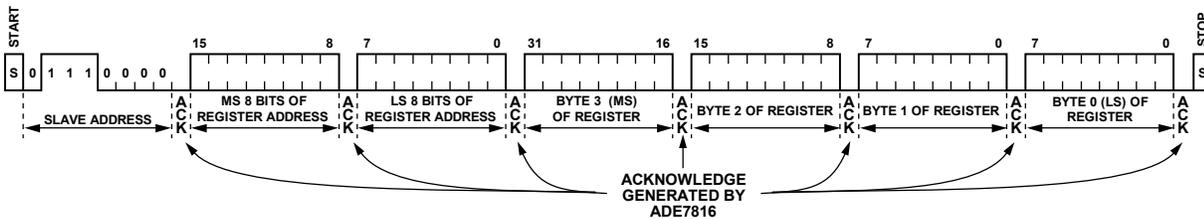
Figure 43. I<sup>2</sup>C Write Operation of a 32-Bit Register
