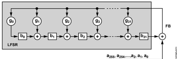
Figure 37. LFSR Generator Used in Checksum Register Calculation
