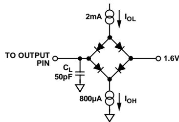
Figure 5. Load Circuit for All Timing Specifications
