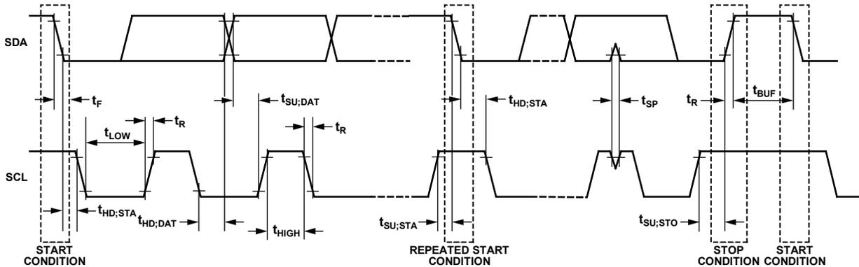
Figure 2. I<sup>2</sup>C-Compatible Interface Timing
