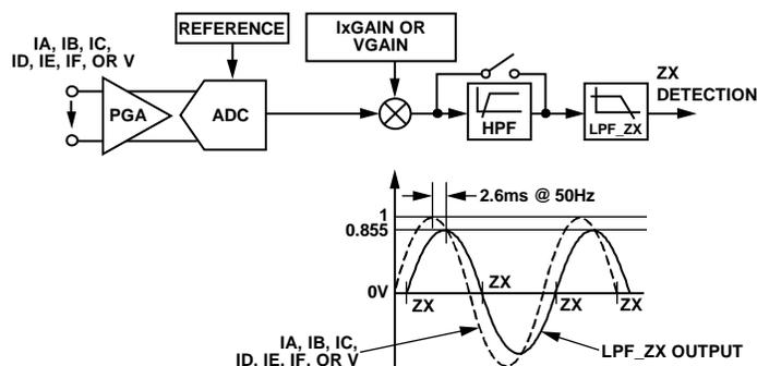
Figure 33. Zero-Crossing Detection
