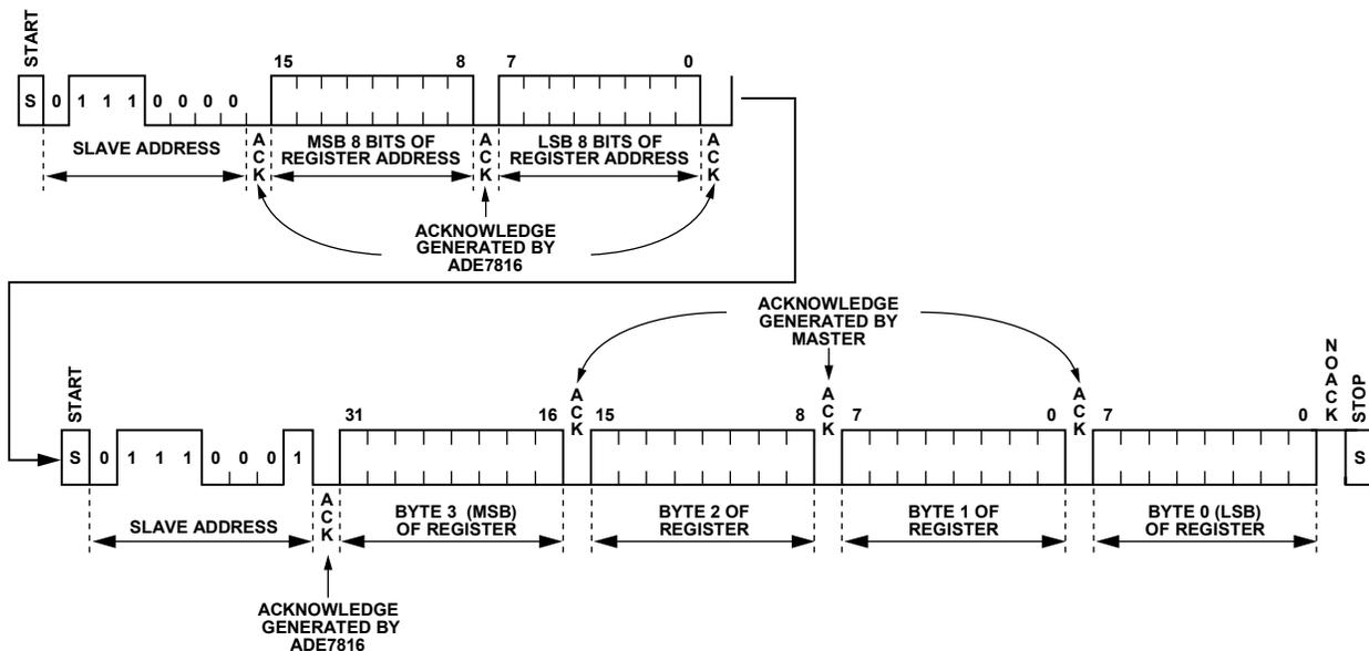
Figure 44. I<sup>2</sup>C Read Operation of a 32-Bit Register
