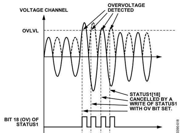
Figure 34. Overvoltage Detection
