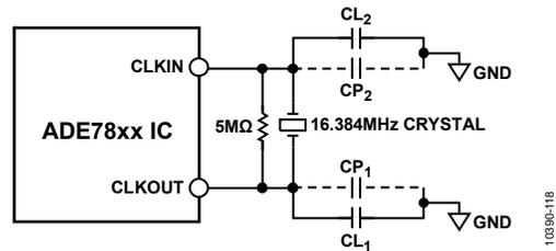
Figure 41. Crystal Circuit
