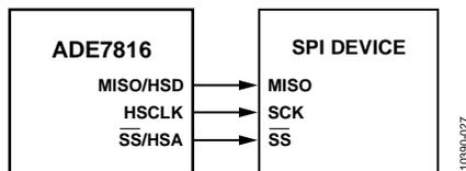
Figure 47. Connecting the ADE7816 HSDC with a SPI
