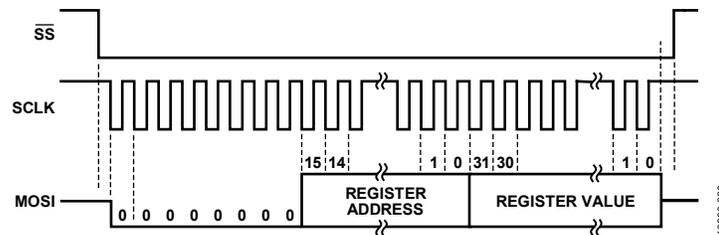
Figure 46. SPI Write Operation of a 32-Bit Register
