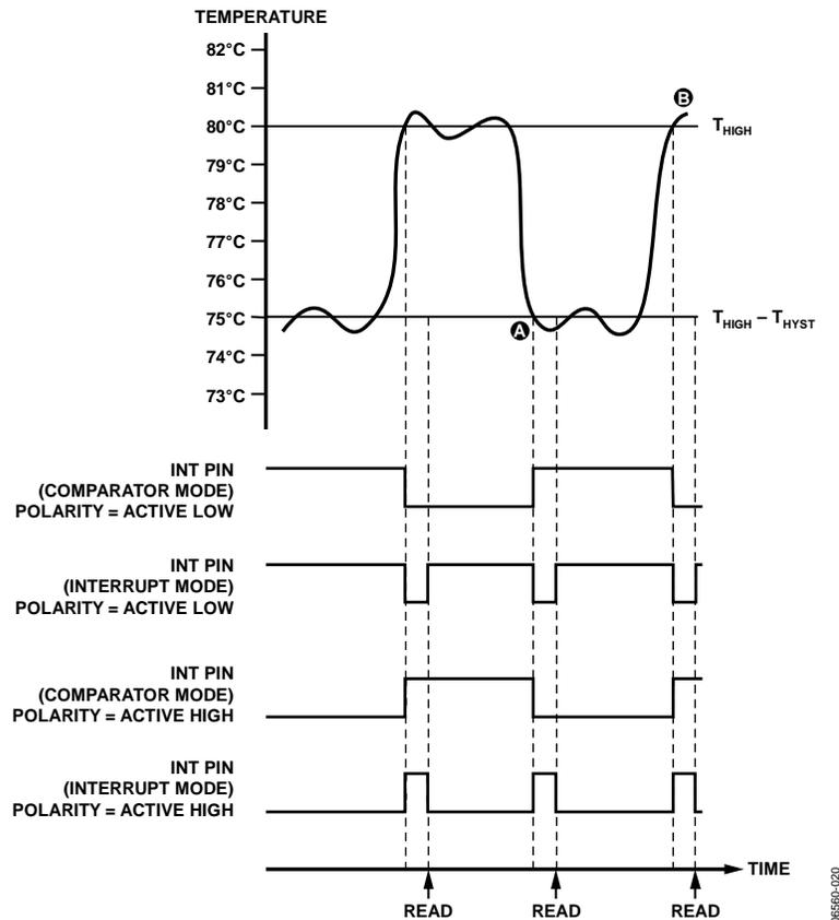
Figure 19. INT Output Temperature Response Diagram for T<sub>HIGH</sub> Overtemperature Events
