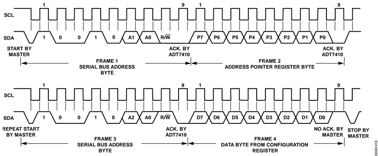
Figure 17. Reading Back Data from the Configuration Register
