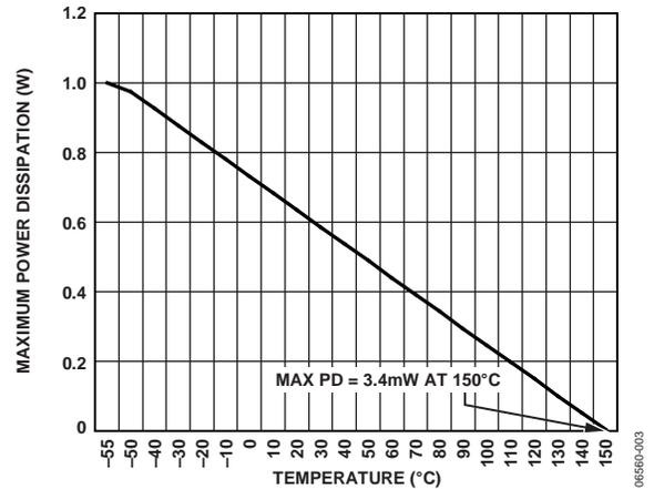
Figure 3. SOIC\_N Maximum Power Dissipation vs. Temperature
