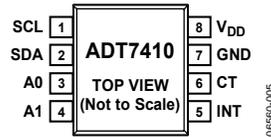
Figure 4. Pin Configuration
