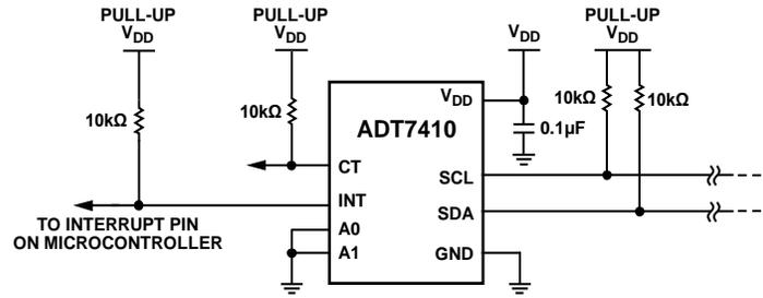
Figure 14. Typical I<sup>2</sup>C Interface Connection
