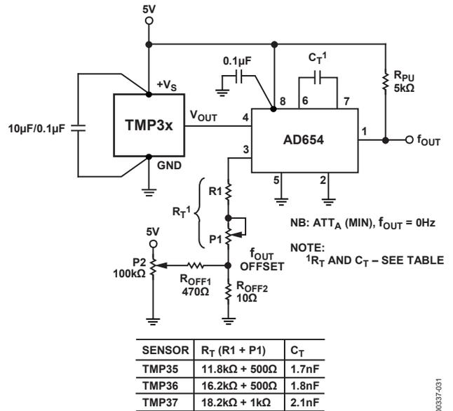
Figure 34. Temperature-to-Frequency Converter
