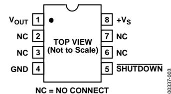
Figure 3. R-8 (SOIC\_N)
