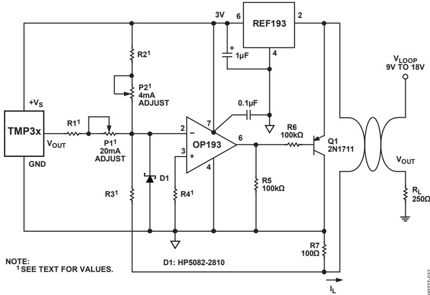
Figure 33. Temperature to 4–20 mA Loop Transmitter
