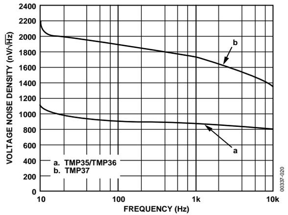
Figure 21. Voltage Noise Spectral Density vs. Frequency
