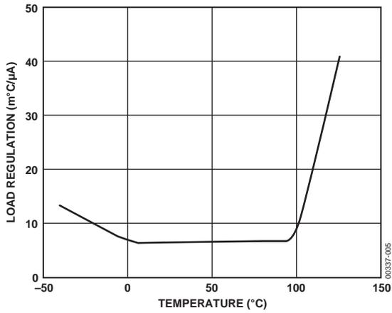
Figure 5. Load Regulation vs. Temperature ( $m^{\circ}C/\mu A$ )
