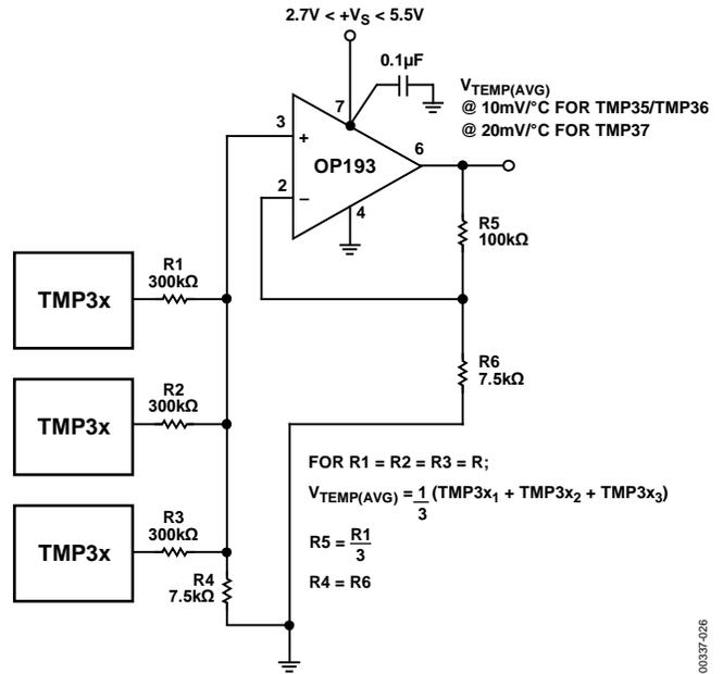
Figure 28. Configuring Multiple Sensors for Average Temperature Measurements
