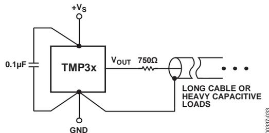
Figure 35. Driving Long Cables or Heavy Capacitive Loads
