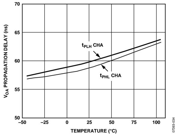
Figure 14. Typical Channel A Propagation Delay vs. Temperature
