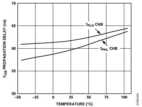
Figure 15. Typical Channel B Propagation Delay vs. Temperature
