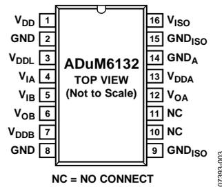
Figure 3. Pin Configuration
