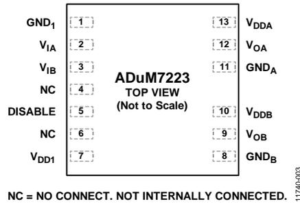
Figure 3. Pin Configuration
