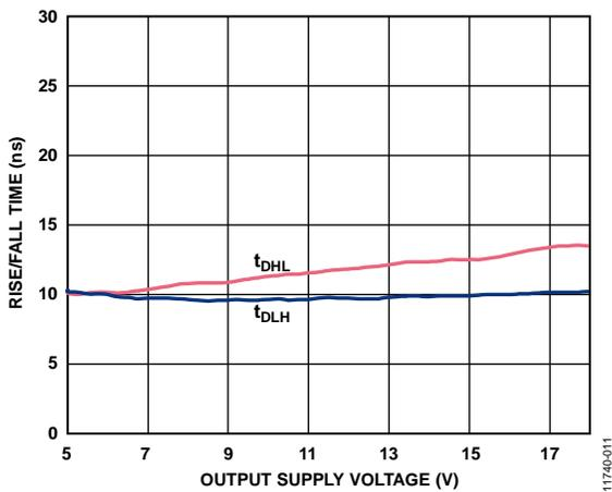
Figure 11. Typical Rise/Fall Time vs. Output Supply Voltage
