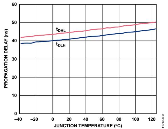
Figure 8. Typical Propagation Delay vs. Junction Temperature
