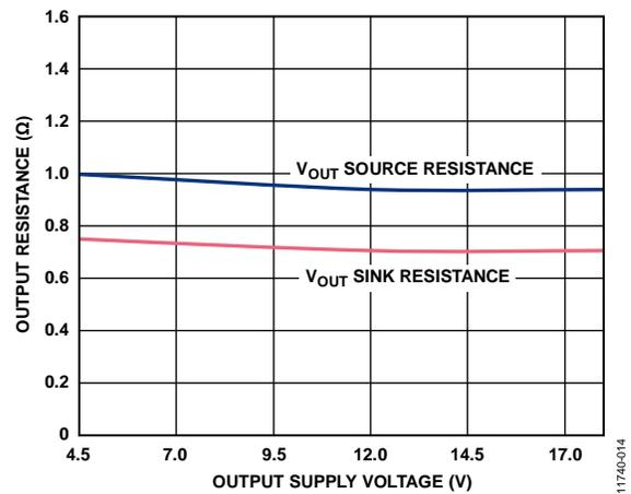
Figure 14. Typical Output Resistance vs. Output Supply Voltage
