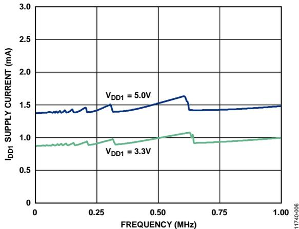
Figure 6. Typical  $I_{DD1}$  Supply Current vs. Frequency
