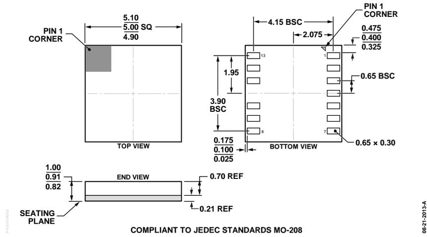
Figure 23. 13-Terminal Land Grid Array [LGA] (CC-13-1)
