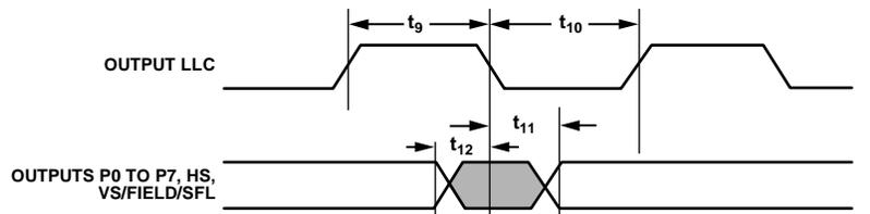
Figure 3. Pixel Port and Control Output Timing
