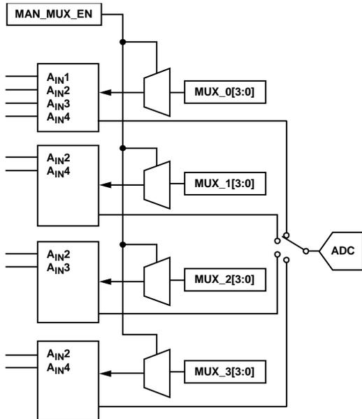
Figure 8. Manual Muxing
