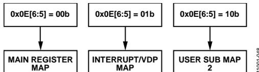
Figure 48. Register Access—Main Register Map, Interrupt/VDP Map, and User Sub Map 2
