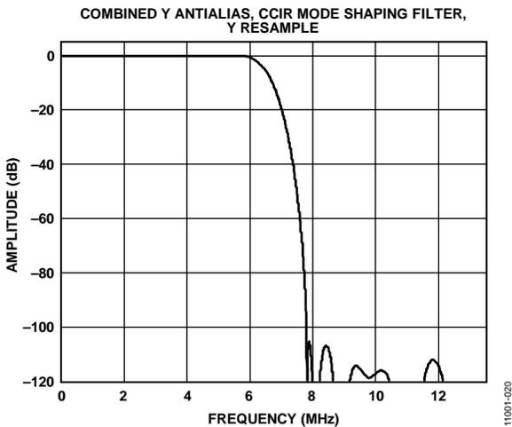
Figure 19. Combined Y Antialias, CCIR Mode Shaping Filter
