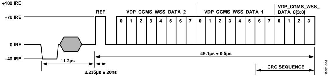
Figure 43. CGMS Waveform
