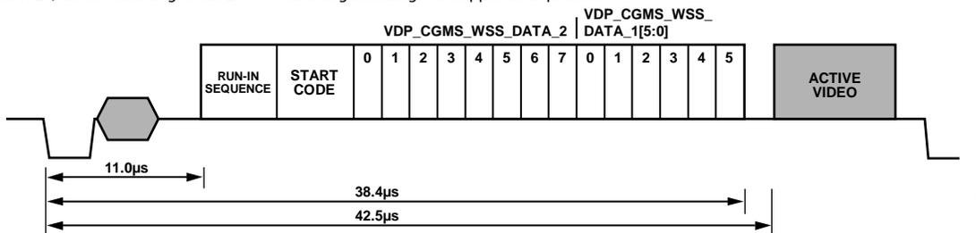
Figure 42. WSS Waveform
