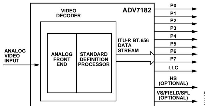
Figure 45. ITU-R BT.656 Output Stage of the [ADV7182](#)
