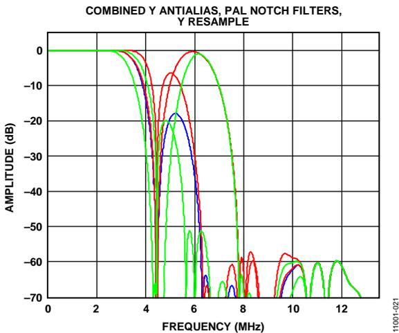
Figure 20. Combined Y Antialias, PAL Notch Filters
