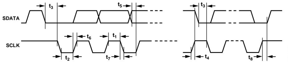
Figure 2. I<sup>2</sup>C Timing
