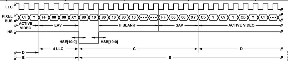
Figure 31. HSYNC Timing
