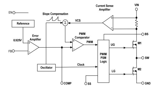
Figure 2. IT76620M Functional Block Diagram
