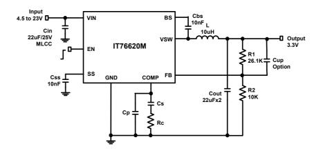
Figure 1. IT76620M Typical Operating Circuit
