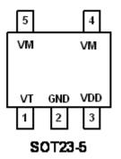
Figure 2. PIN Configuration
