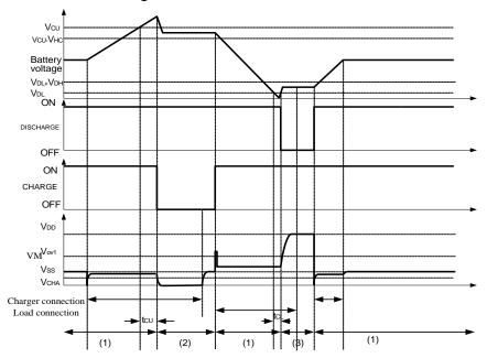
Figure 5-1 Overcharge and Overdischarge Voltage Detection
