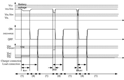
Figure 5-2 Overdischarge Current Detection
