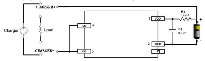
Fig 6 XB5350G in a Typical Battery Protection Circuit
