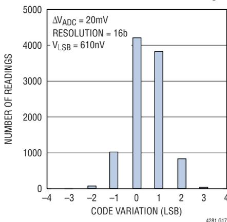
**12-Bit GPIO ADC Noise Histogram**
