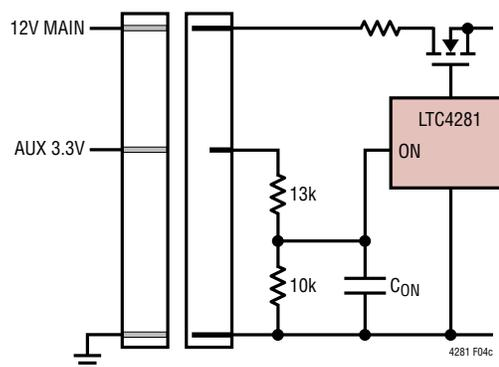
(c) ON Pin Sensing of AUX Supply ON
