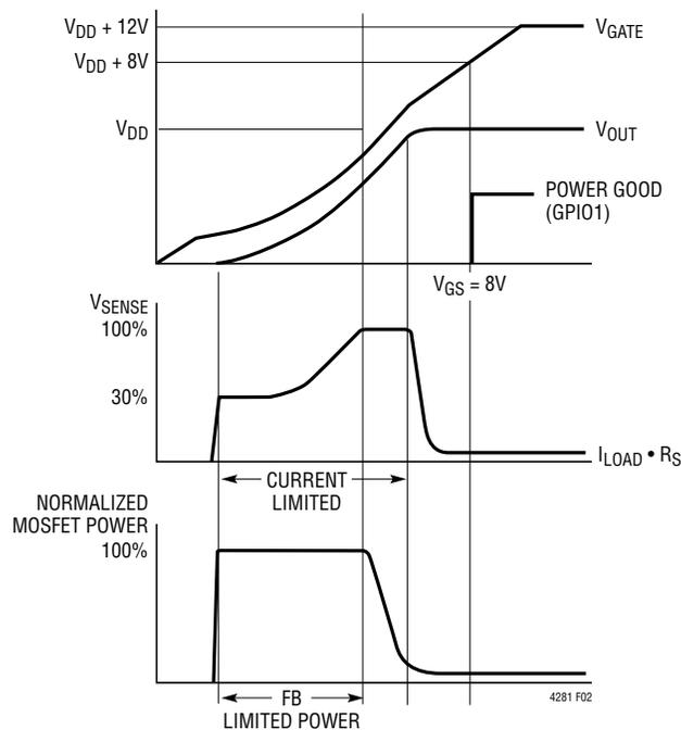
Figure 2. Power-Up Waveforms
