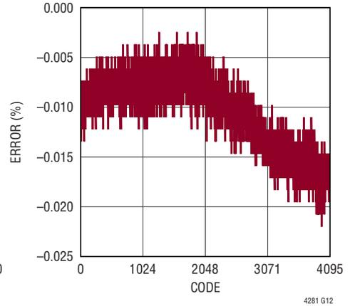
**ADC Integral Non-Linearity vs Code (INL vs Code)**
