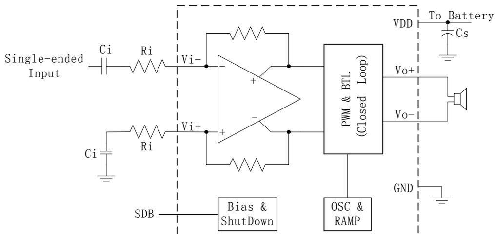
Figure 4. BL6306 Application Schematic With Single-Ended Input
