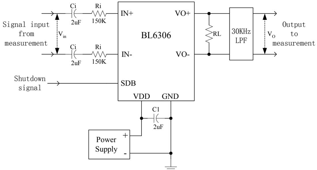
Figure 5. BL6306 test set up circuit
