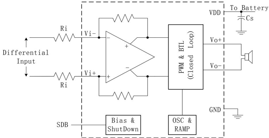
Figure 2. BL6306 Application Schematic With Differential Input
