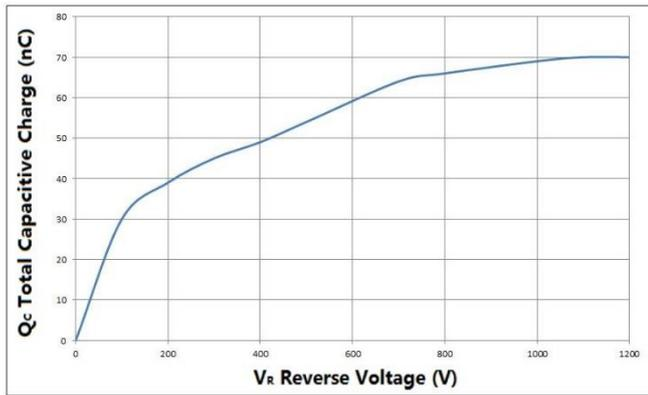
Fig. 3 Total Capacitance Charge vs. Reverse Voltage
