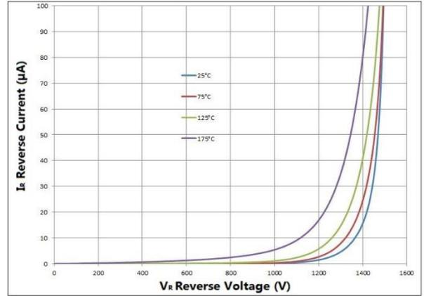
Fig. 2 Reverse Characteristics
