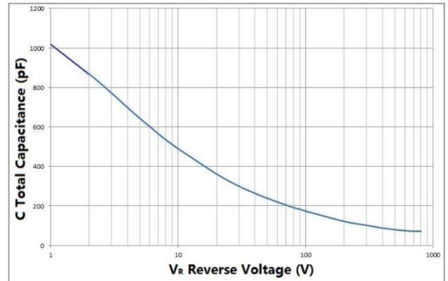
Fig. 4 Total Capacitance vs. Reverse Voltage
