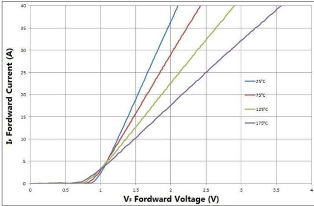
Fig. 1 Forward Characteristics
