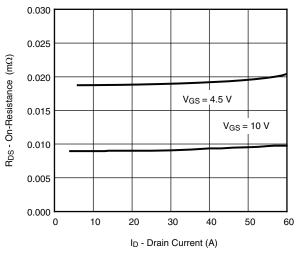
On-Resistance vs. Drain Current
