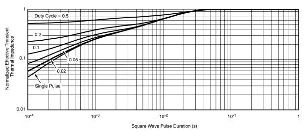
Normalized Thermal Transient Impedance, Junction-to-Case
