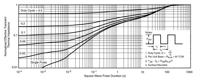
Normalized Thermal Transient Impedance, Junction-to-Ambient
